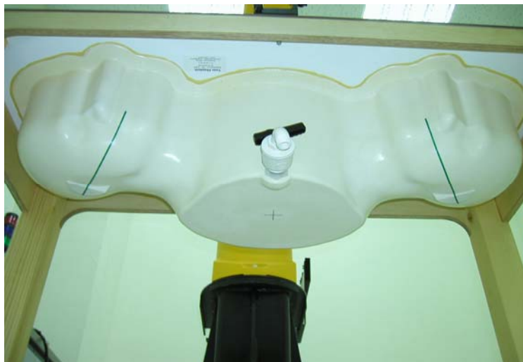
Fig. 5.4 Bottom View of Twin Phantom
