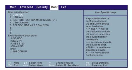
The bootable devices will be automatically detected during POST and shown here, allowing you to set the sequence that the BIOS uses to look for a boot device from which to load the operating system. A brief description of keyboard usage is listed next:
