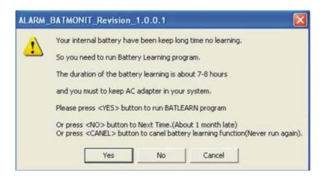
Click **Yes** to run the **Battery Learning** program's recalibration function to fully charge the battery pack, discharge it completely, then fully charge it again.
