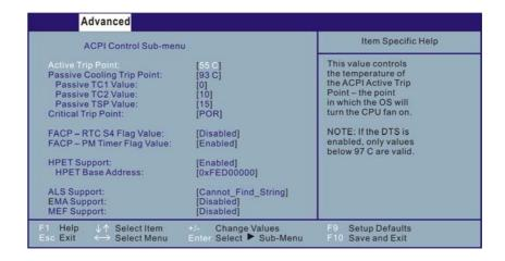
**Active Trip Point** controls the temperature of ACPI Active Trip Point – the point in which OS will turn the CPU fan on.
