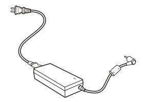
The AC adapter serves as a converter from AC (Alternating Current) to DC (Direct Current) power because your computer runs on DC power, but an electrical outlet usually provides AC power. It also charges the battery pack when connected to AC power.
