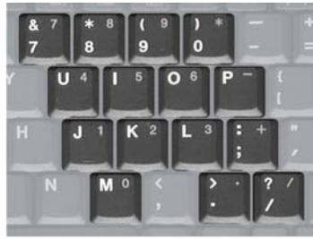
Numeric keys facilitate entering of numbers and calculations. When Num Lock is on, the numeric keys are activated; meaning you can use these keys to enter numerals.
