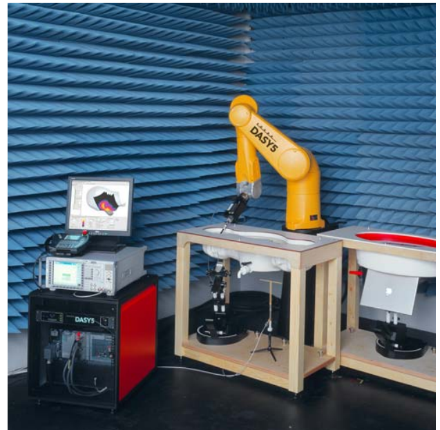
Fig. 5.2 Probe Setup on Robot
