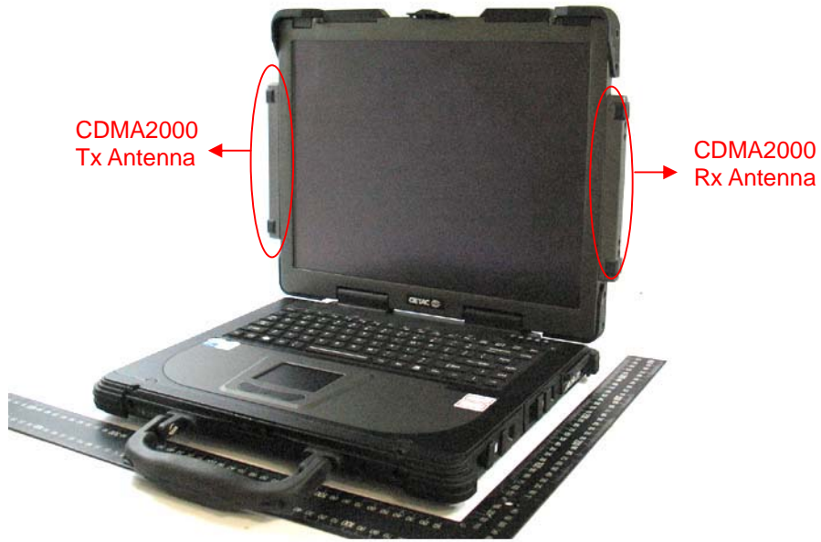
CDMA2000 Antenna Location
