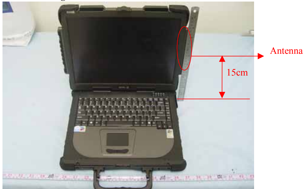
Fig. 9.4 Antenna Position for M230-5
