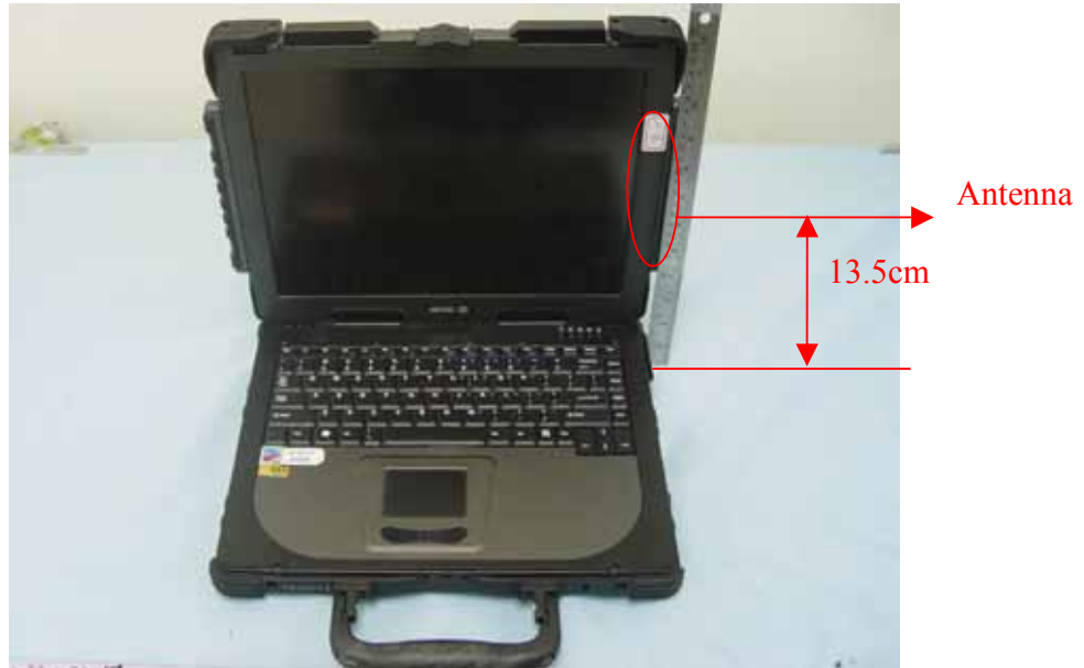
Fig. 9.3 Antenna Position for M230-4
