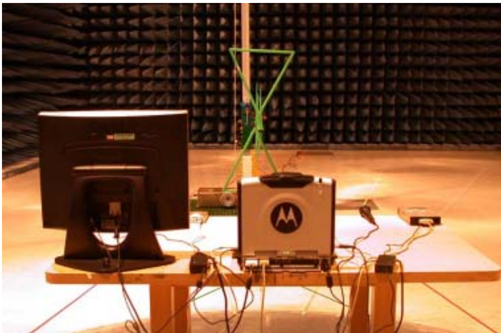
The Back View of Highest Radiated Set-up For EUT
