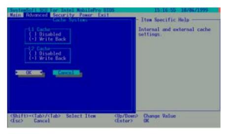
The "Cache Systems" item Write Back (enables) the cache of your system: L1 cache (internal cache of CPU) and L2 cache (external 256KB or 512KB cache). The cache feature enhances system performance because the most
