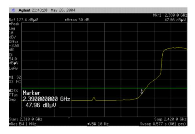
Detector mode: Peak Polarity: Horizontal
