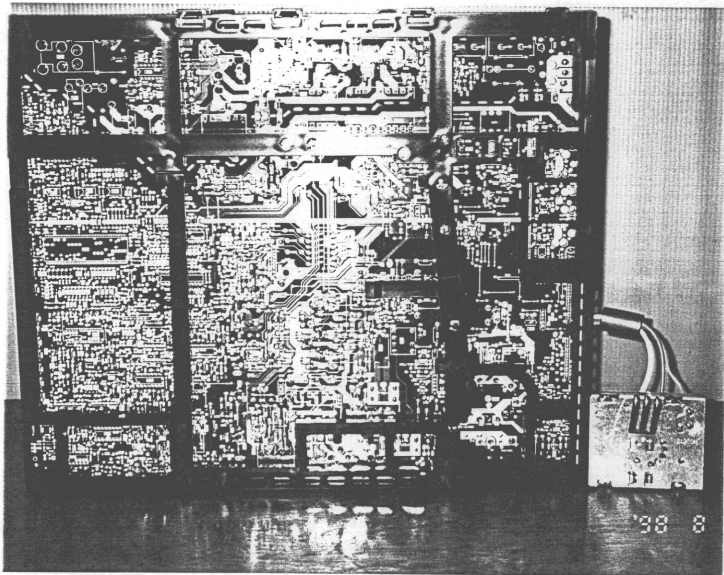
**Photograph No. 10: Main board- solder side**
