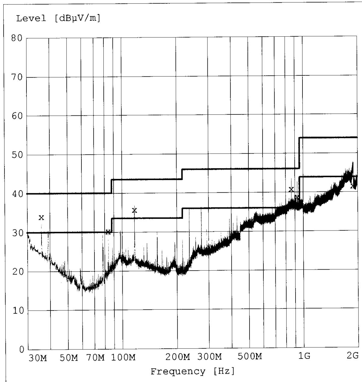
**Measurement of Radiated E-Field Emissions over the
