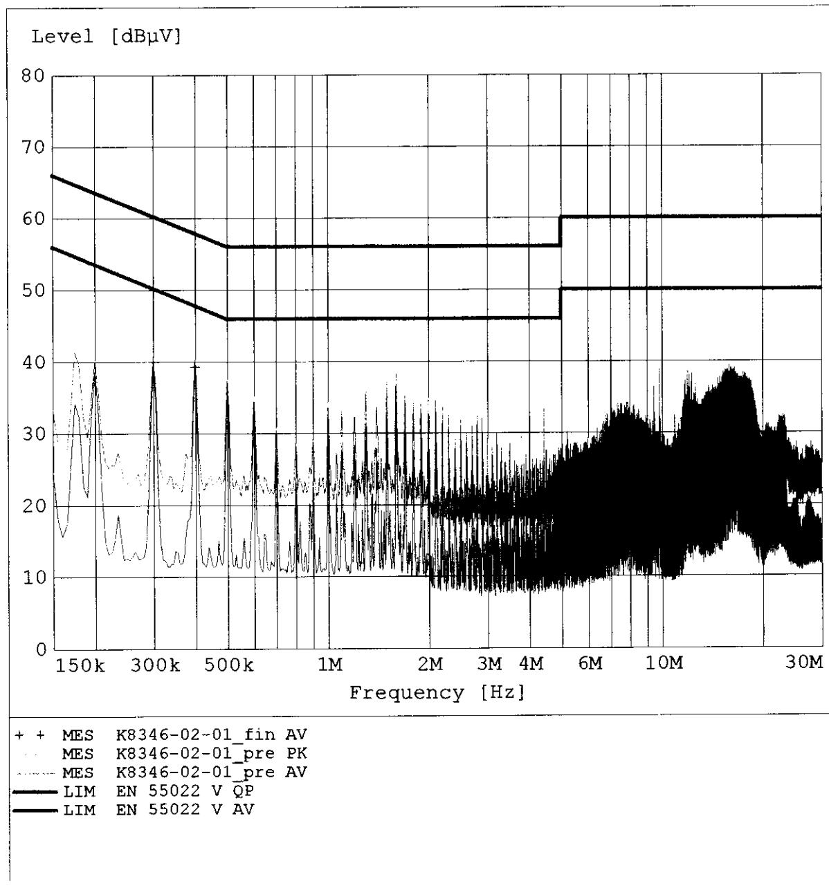
**Measurement of Power Line Conducted Emissions
