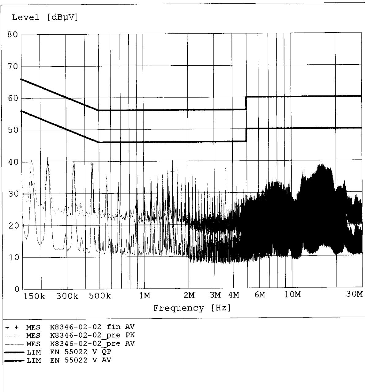
**Measurement of Power Line Conducted Emissions
