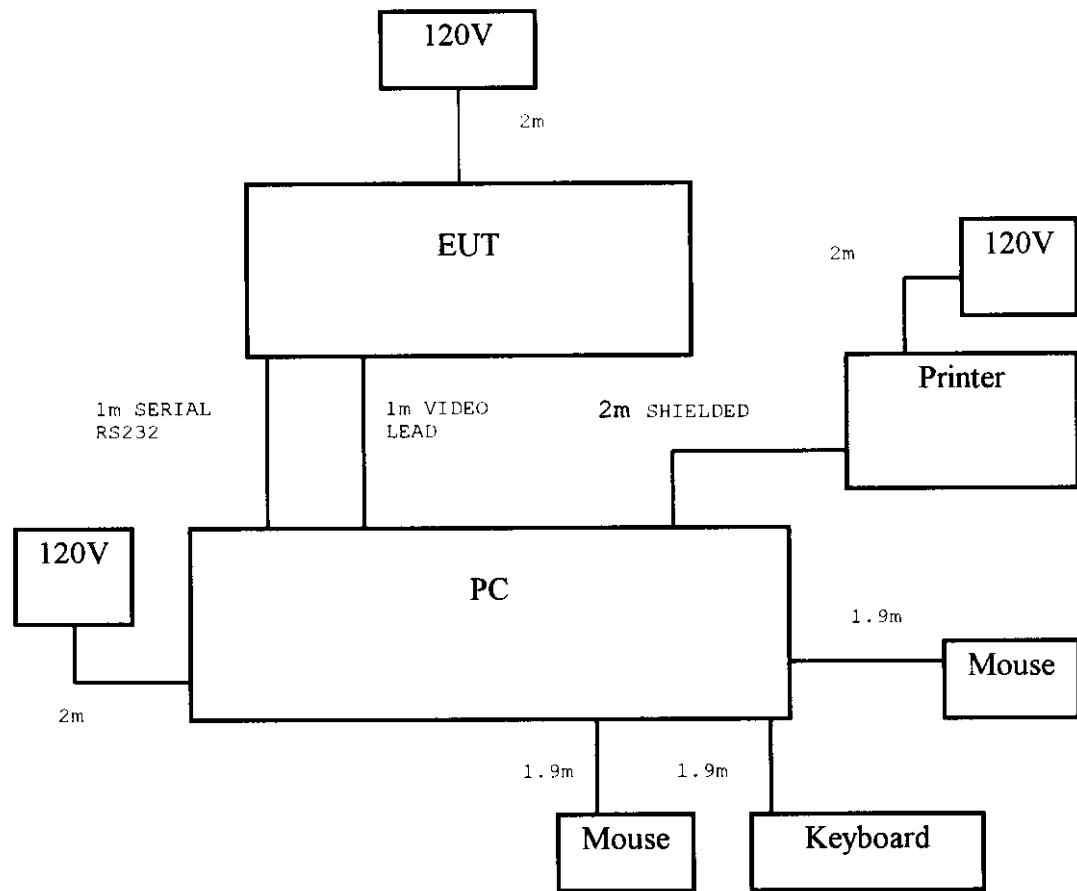
Note 1: Both serial lead and video lead were standard Hitachi Home Electronic cable with ferrite on either end.
