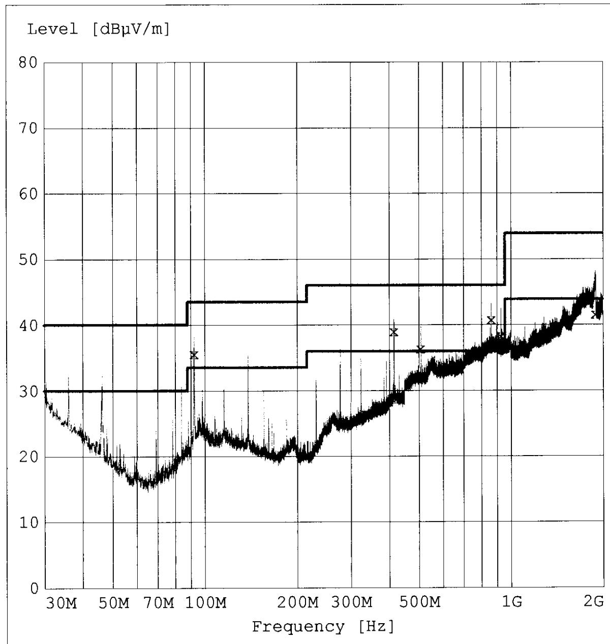
**Measurement of Radiated E-Field Emissions over the
