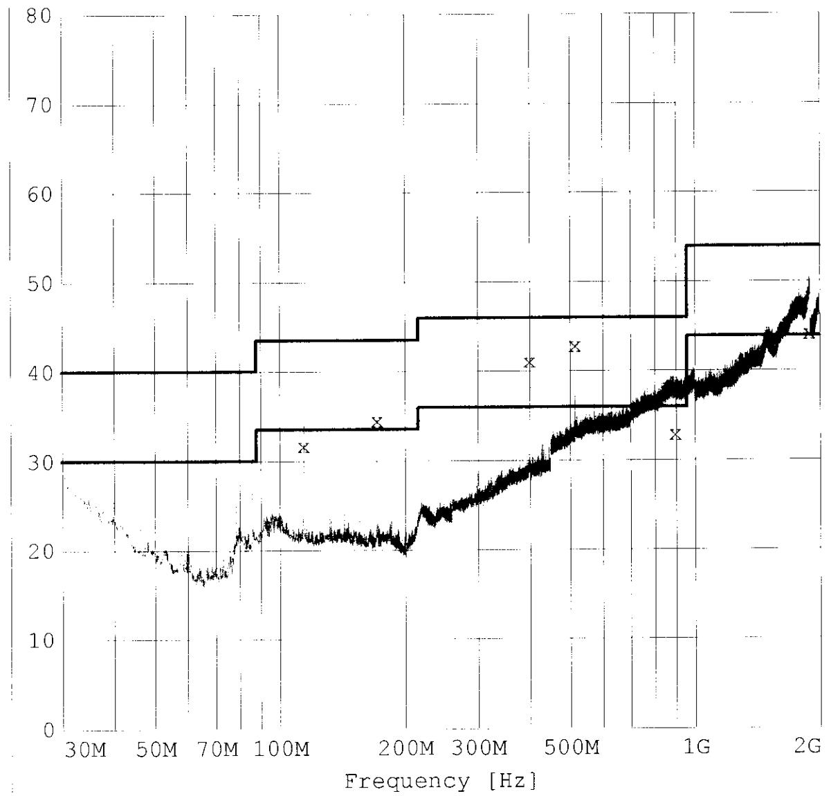
**Measurement of Radiated Emissions over frequency
