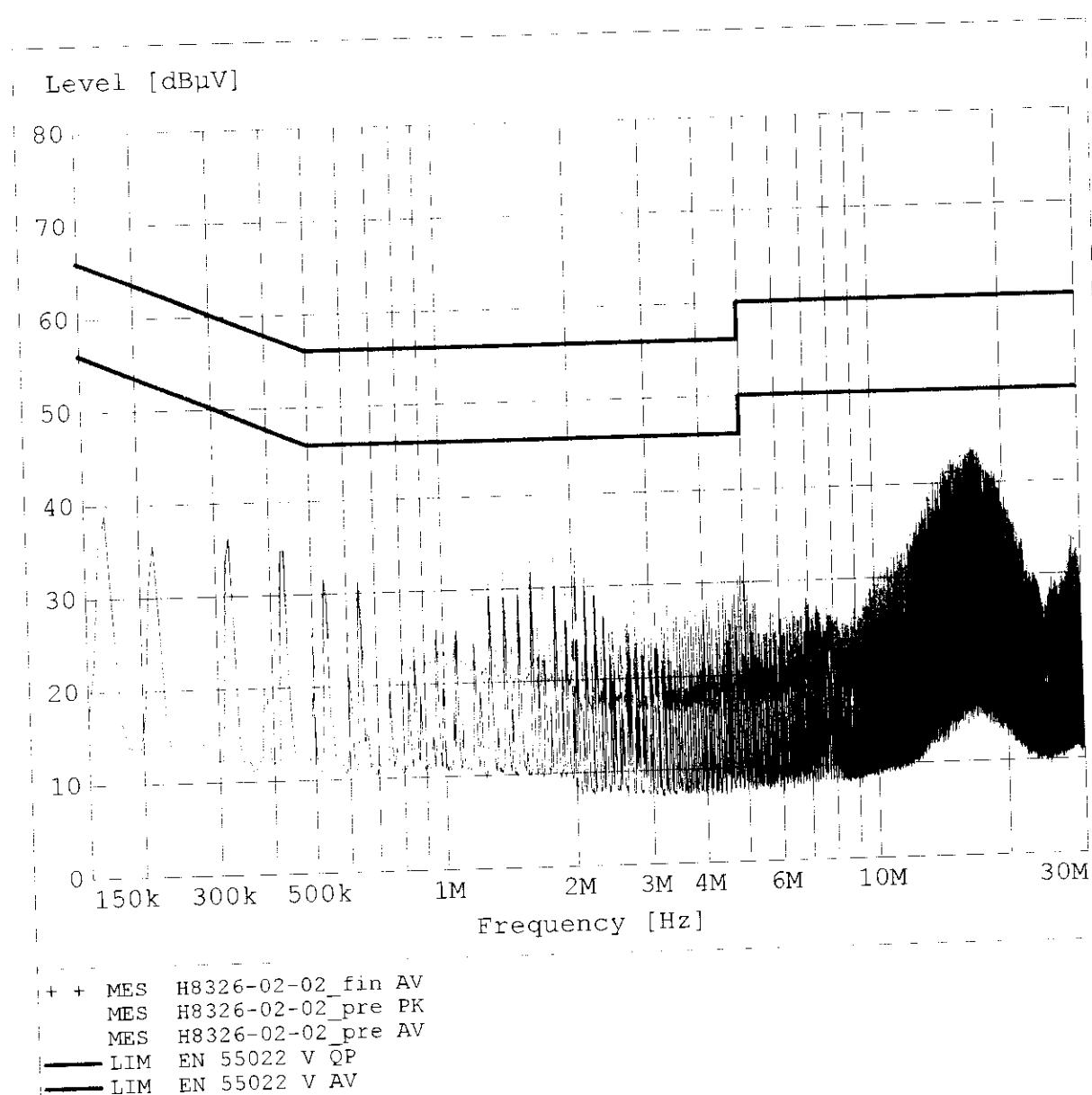
**Measurement of Mains Terminal Disturbance Voltage
