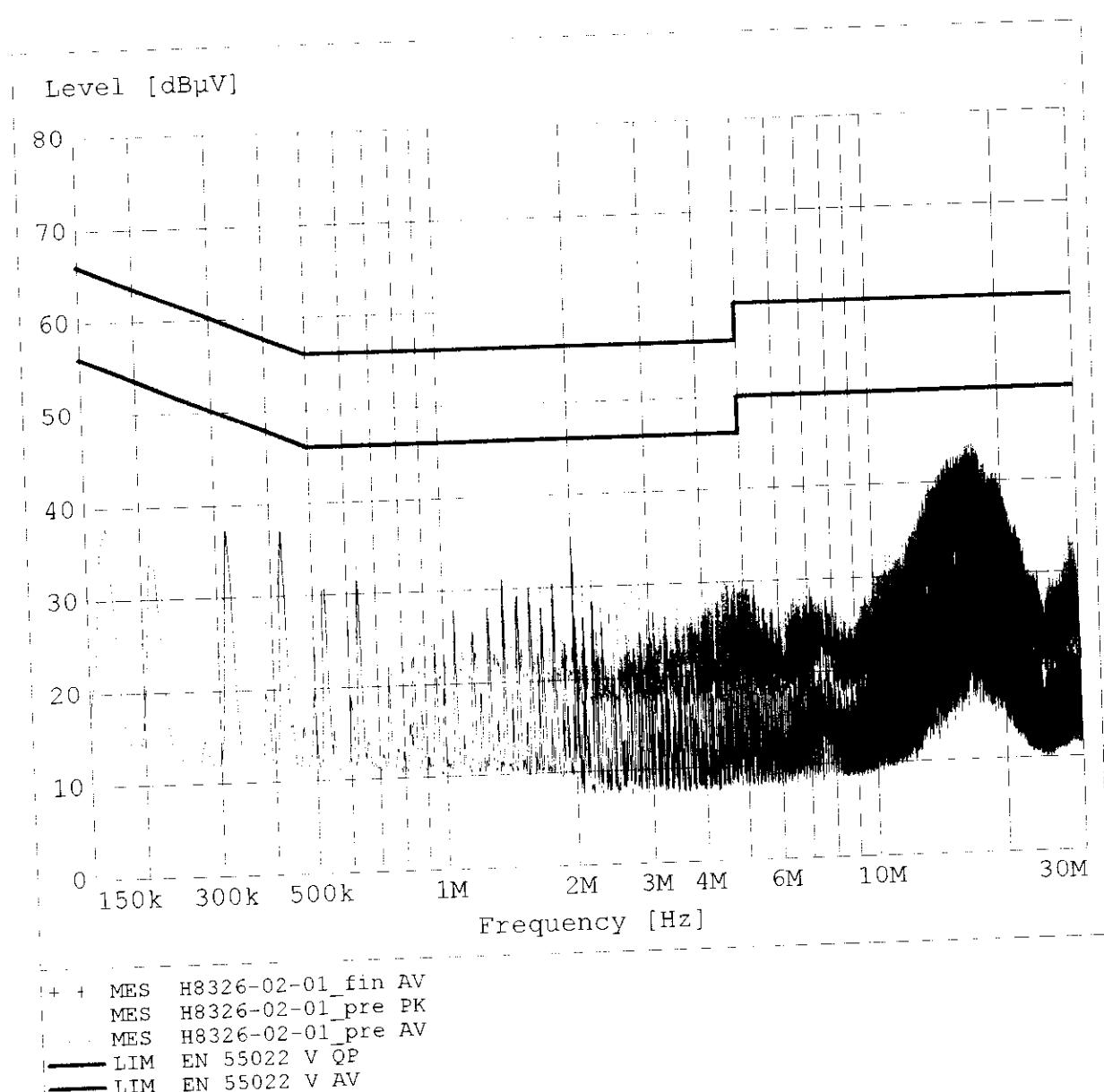
**Measurement of Mains Terminal Disturbance Voltage
