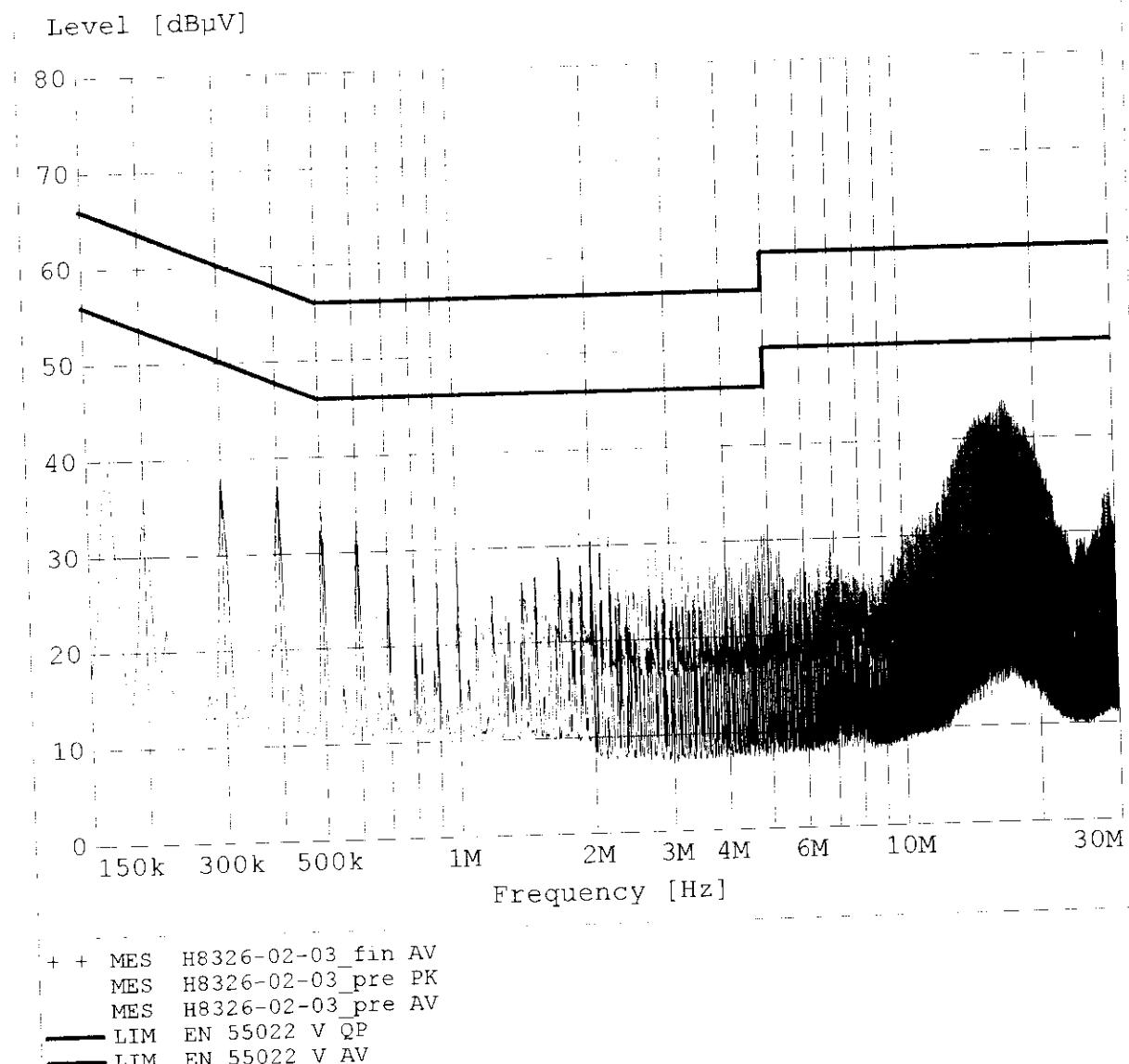
*Measurement of Radiated Emissions over frequency*
