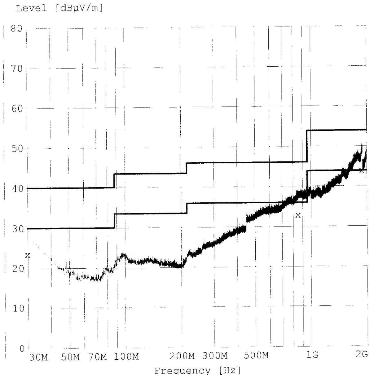
*Measurement of Radiated Emissions over frequency*
