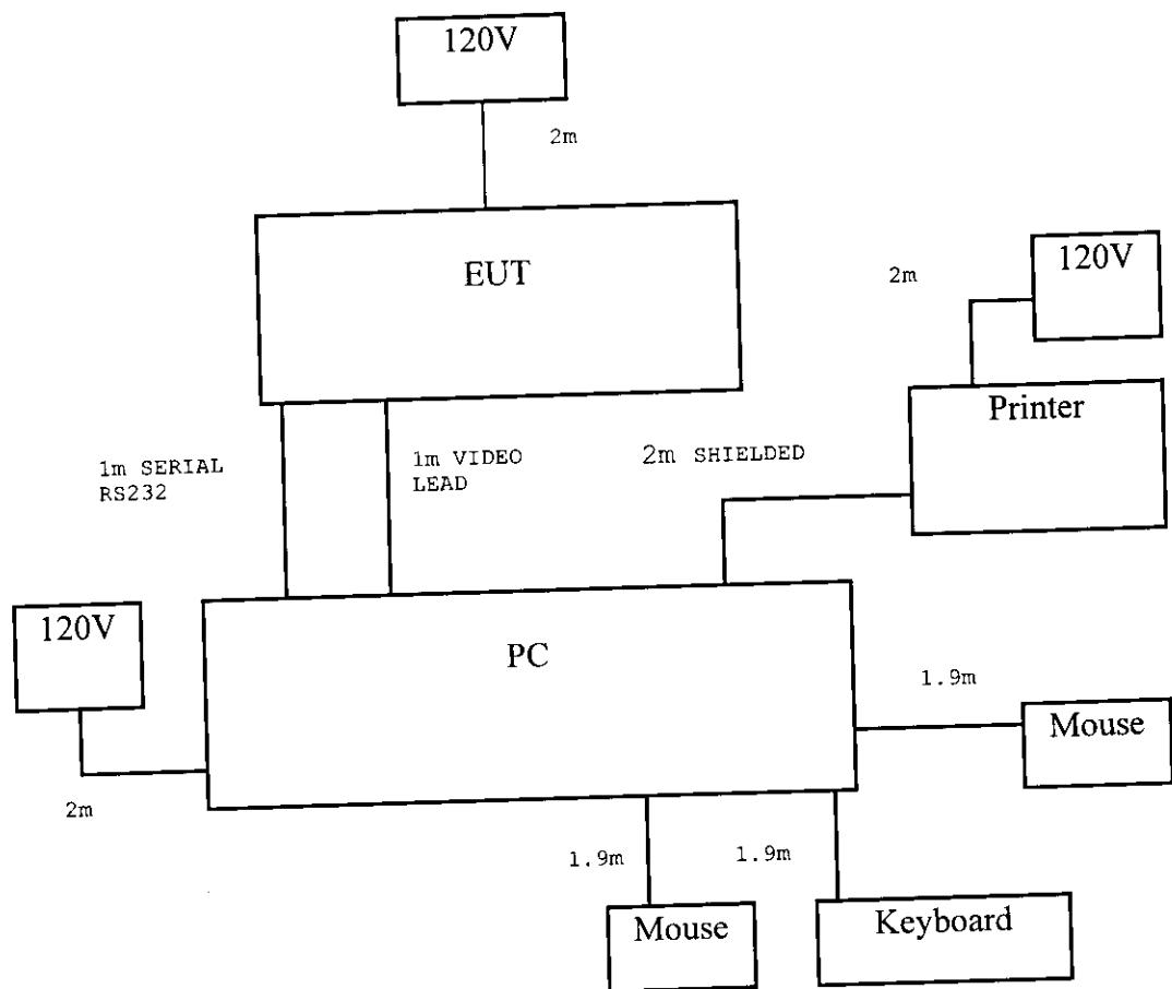
Note 1: Both serial lead and video lead were standard Hitachi Home Electronic cable with ferrite on either end.
