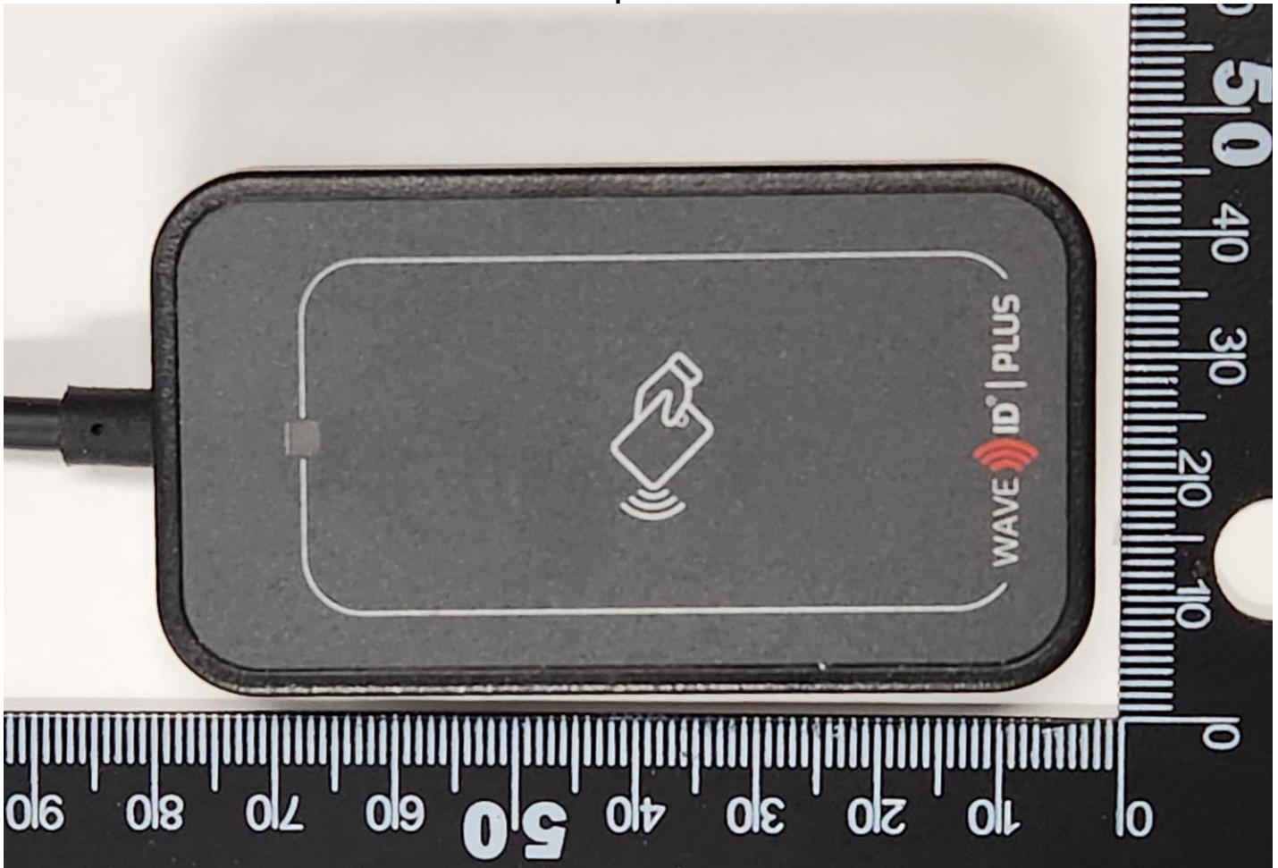
The plastic enclosure measures 3 1/2 inches long x 2 inches wide x 5/8 inches thick
