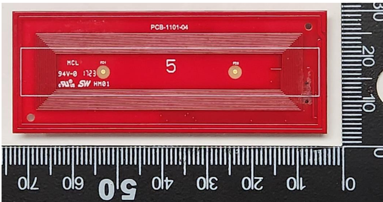
Antenna PCB Bottom
