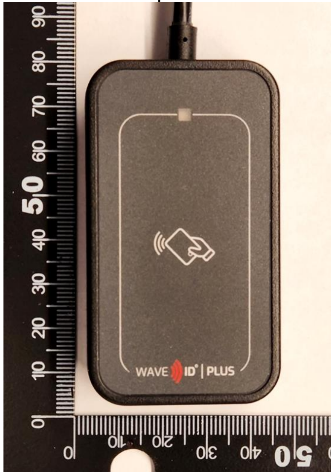
The plastic enclosure measures 3 1/2 inches long x 2 inches wide x 5/8 inches thick
