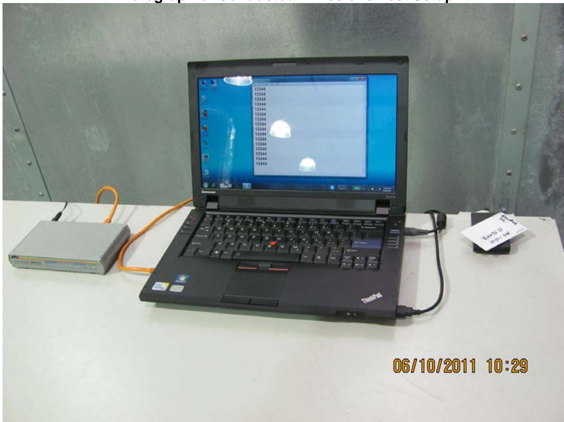
Photograph of Conducted Emissions Test Setup
