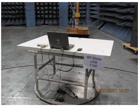
Photographs of Magnetic Radiated Emissions Test Setup
