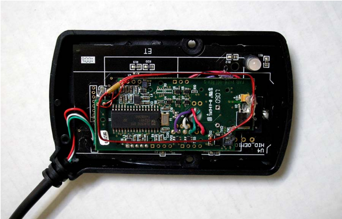
Photograph of Component side of RF PCB showing Antenna
