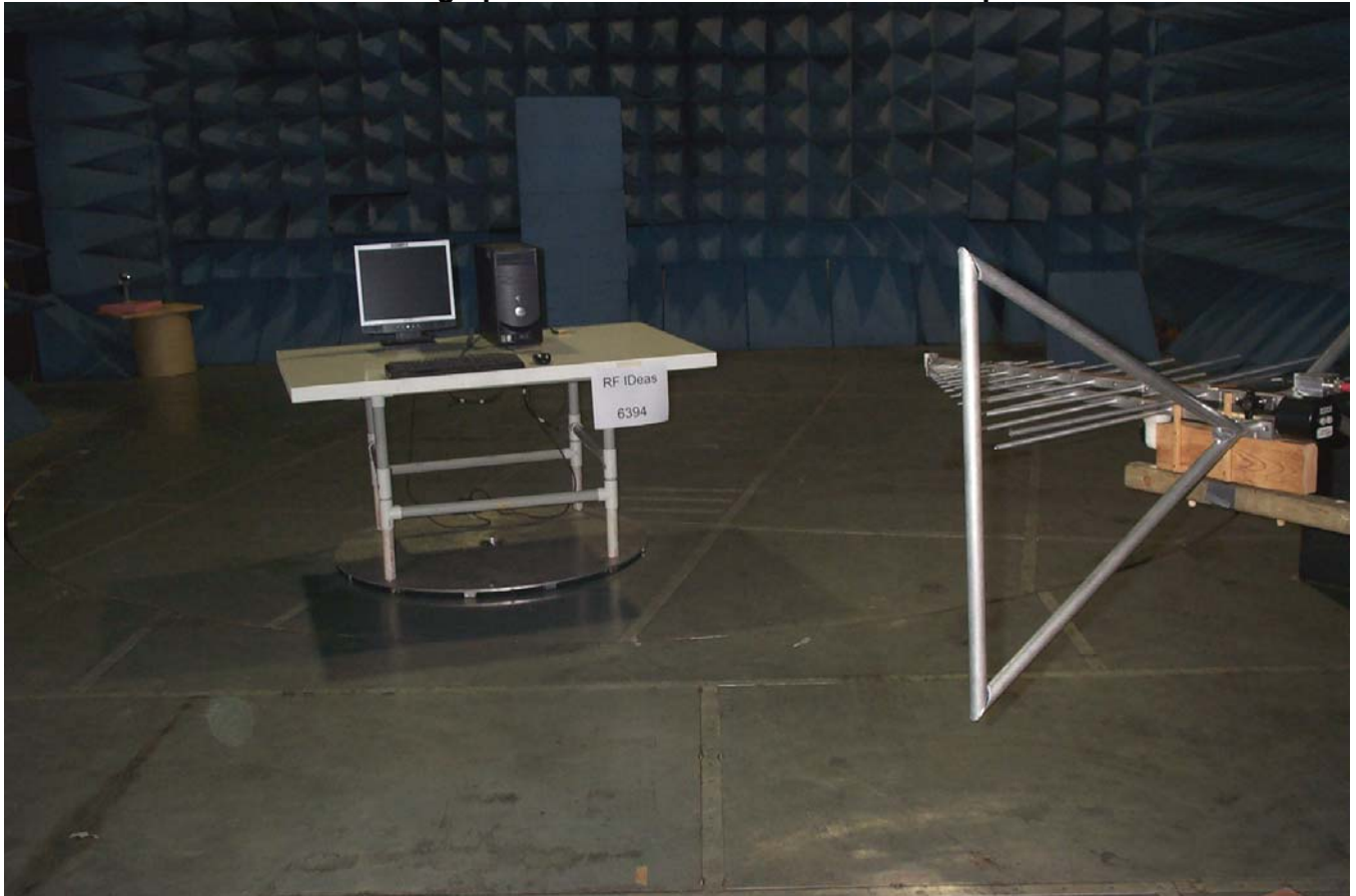
Photograph of Radiated Emissions Test Setup
