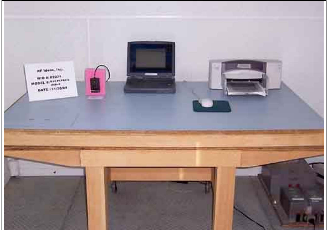
Mains Conducted Emissions - Front View
