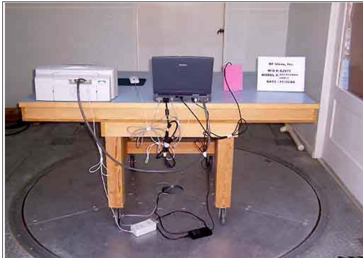
Radiated Emissions - Back View
