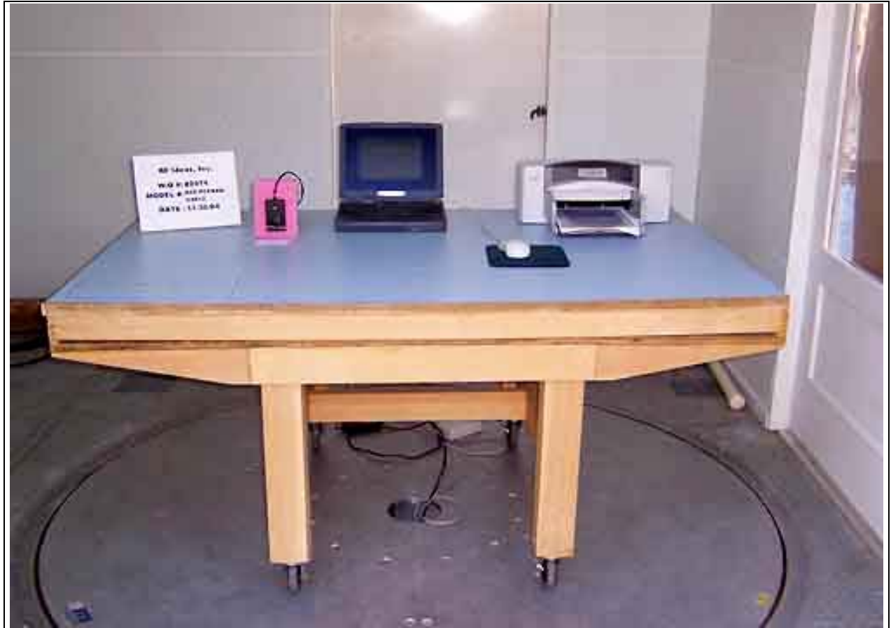
Radiated Emissions - Front View
