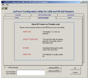
There are several bits constructed together which make up the data sent from the proximity token to the pcProx reader. The pcProx reader reads all bits for any format card produced.
