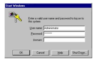
As with the Change Password operation described above, the user first makes sure the cursor is in the Password field. Once the cursor is located, the user waves the proximity token to fill in the *Password* field. If the password is made up of the card data + a user supplied PIN, you will need to add this PIN prior to pressing the ENTER key.
