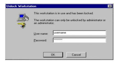
Once the cursor is in the Password field, the user may safely wave their proximity token over the pcProx reader and the field is stuffed with the password. The user may finish off the operation by pressing the ENTER key, or the reader may be configured to add the ENTER keystroke as an appended keystroke.
