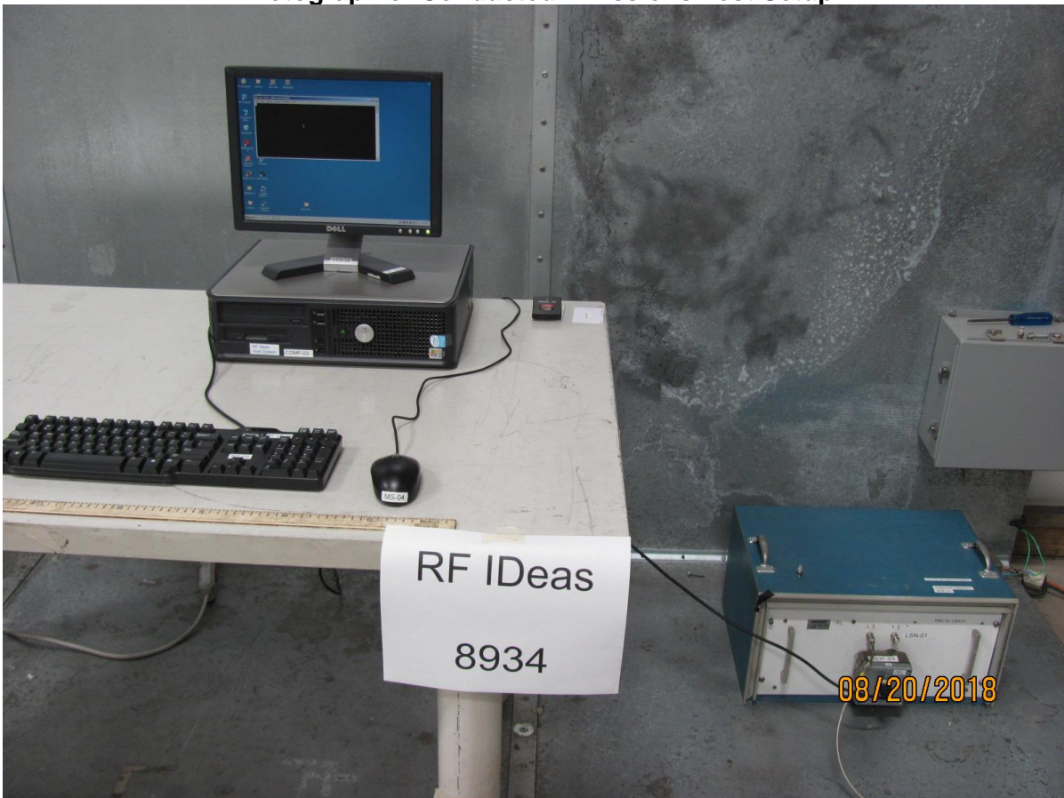
Photograph of Conducted Emissions Test Setup
