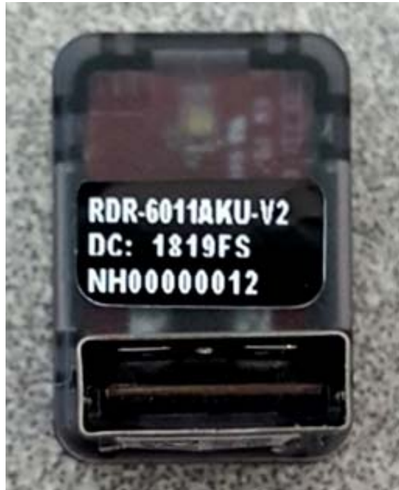
Label Type: Brady P/N: THT-96-473-10 Color: Black with White text Size of Label: 0.275" X 0.5" Adhesive: Permanent Model Numbers will be actual number as shown Below
