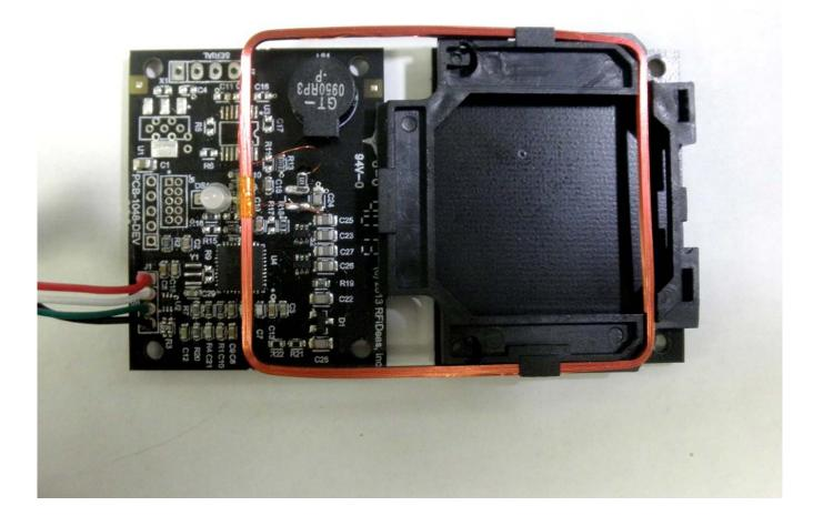
Component Side: Antenna removed
