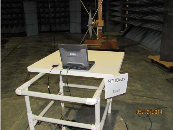
Photographs of Radiated Emissions Test Setup
