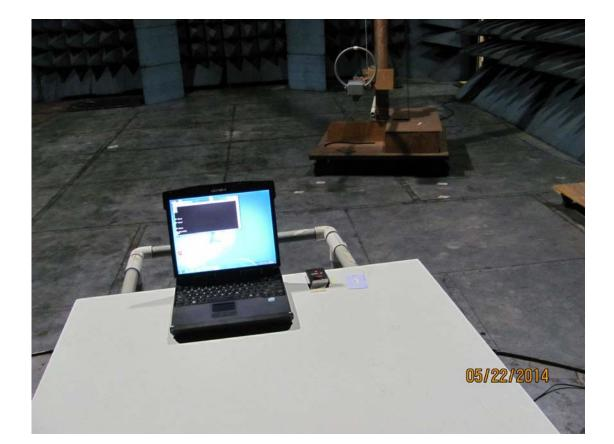
Photograph of Conducted Emissions Test Setup
