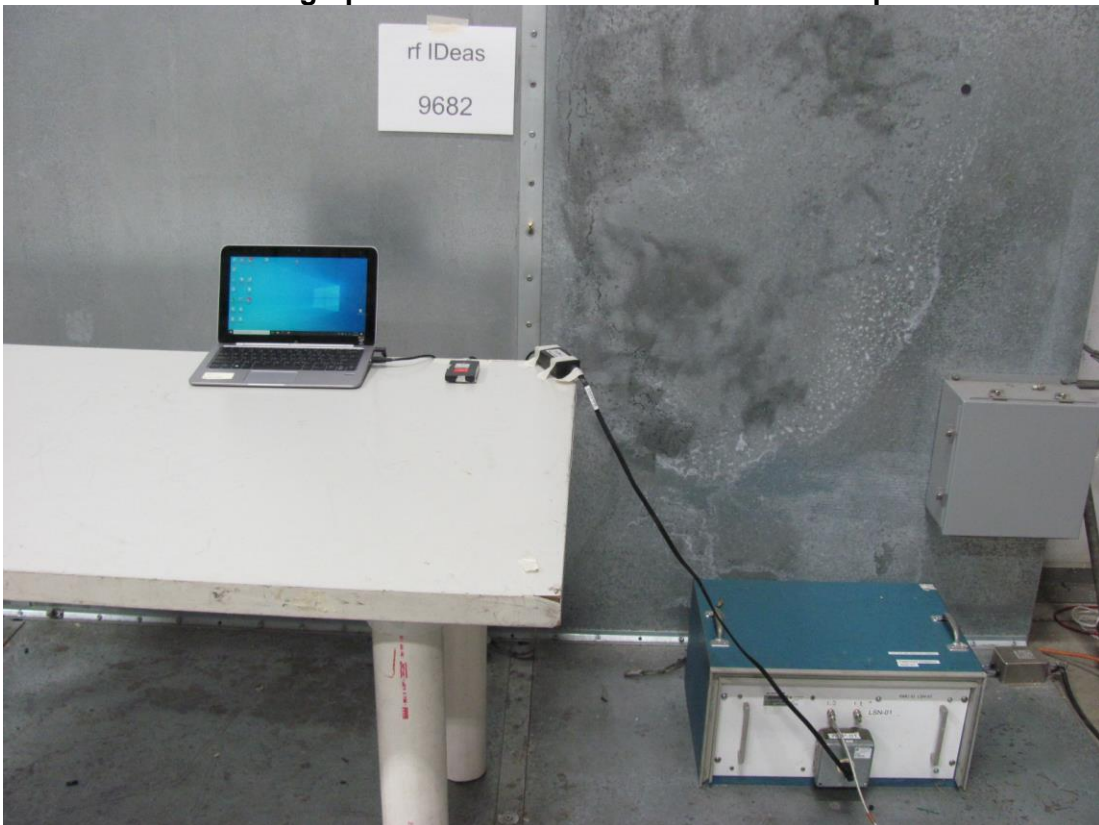
Photograph of Conducted Emissions Test Setup
