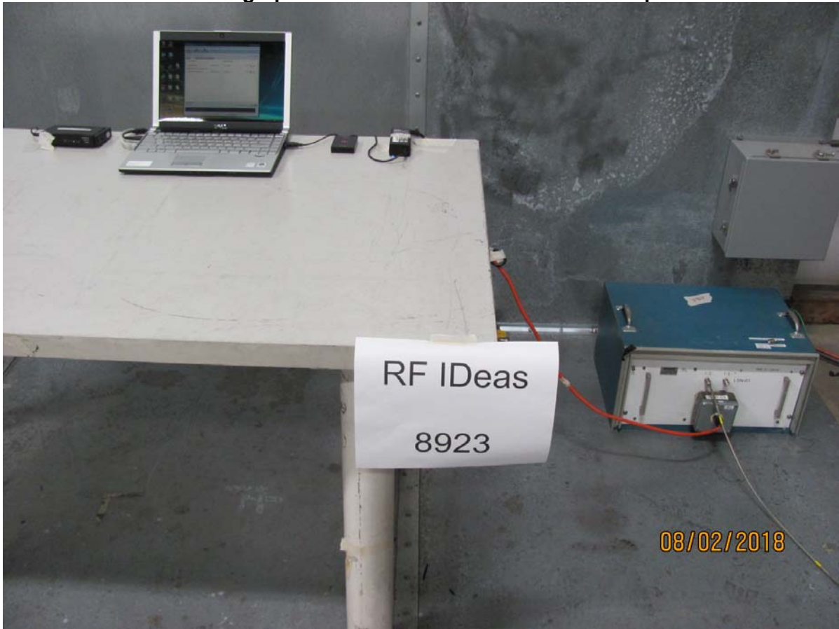
Photograph of Conducted Emissions Test Setup
