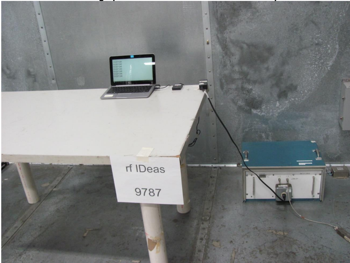
Photograph of Conducted Emissions Test Setup
