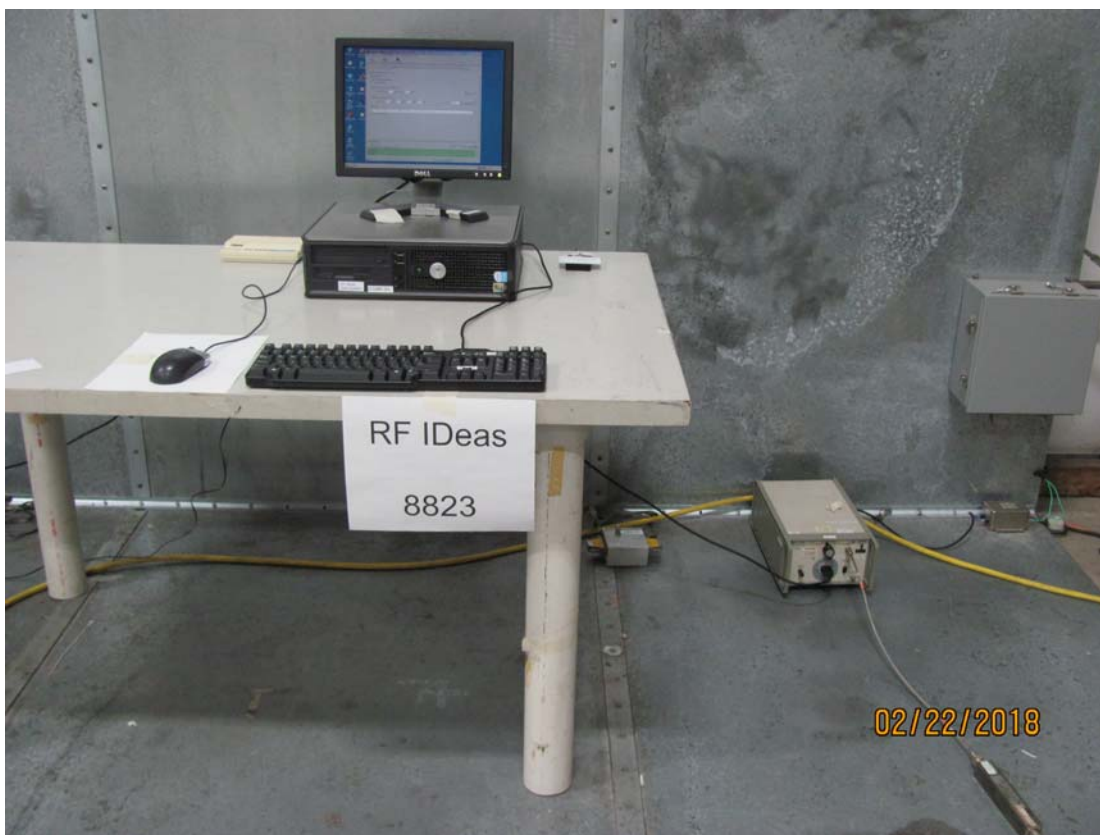
Photograph of Conducted Emissions Test Setup
