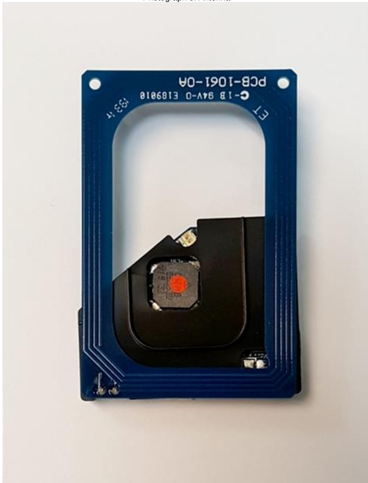
Photograph of Antenna
