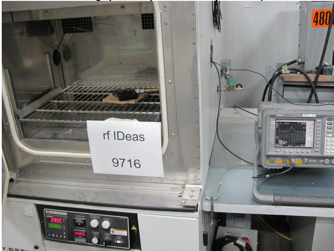
Photograph of Temperature Stability Test Setup
