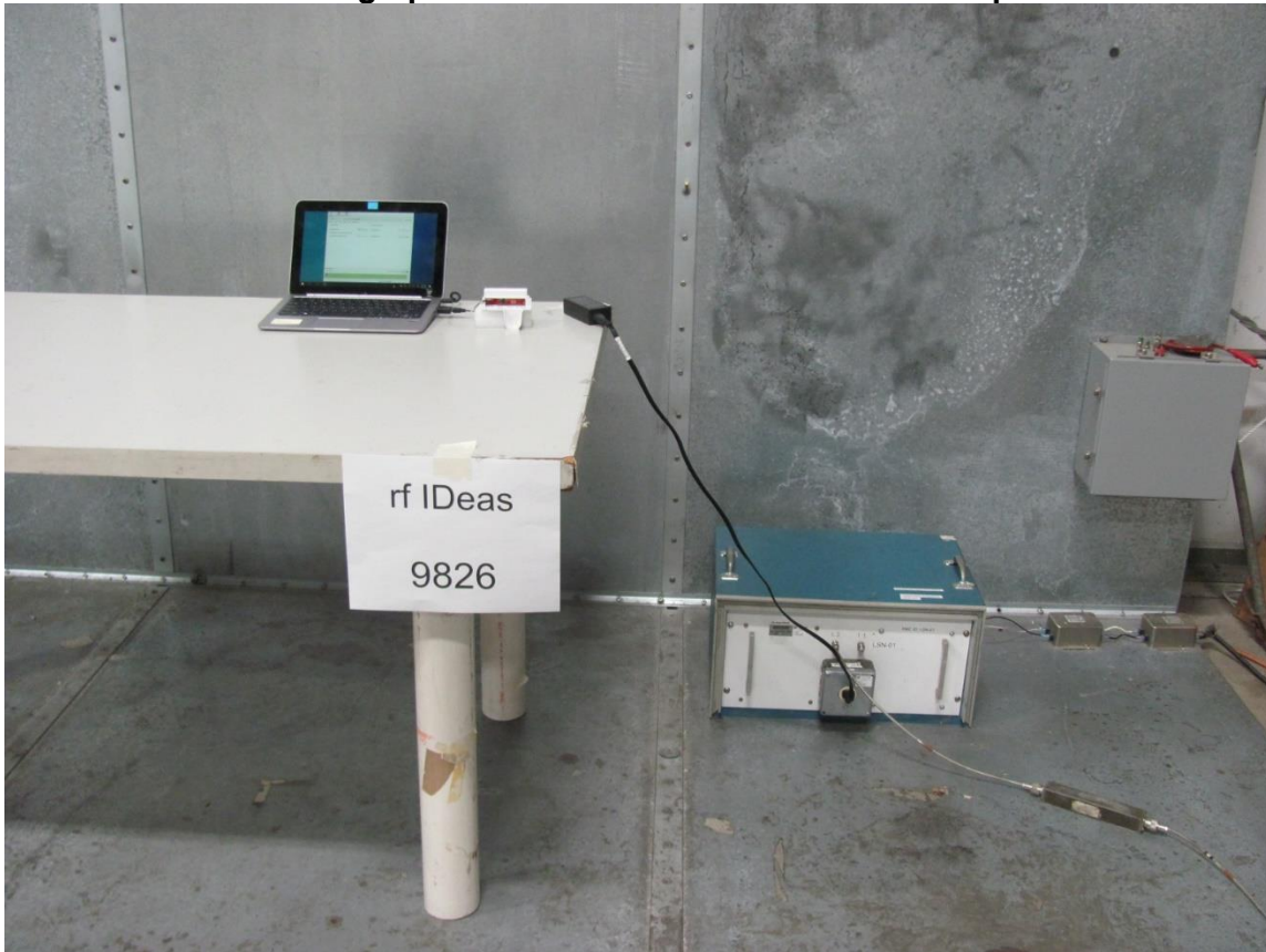
Photograph of Conducted Emissions Test Setup
