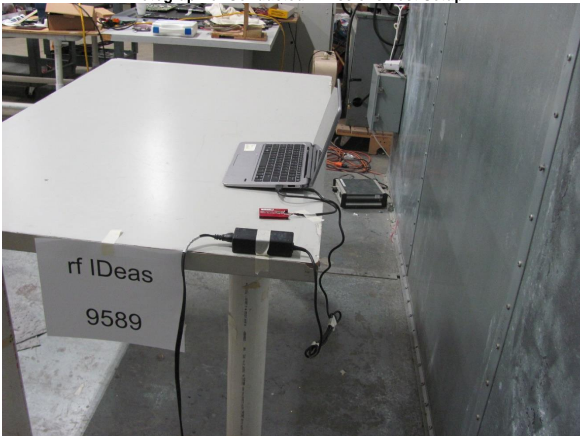
Photograph of Conducted Emissions Test Setup
