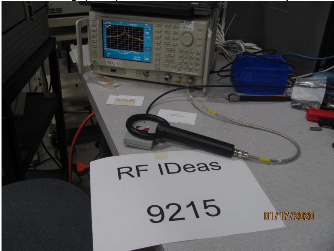
Photograph of Spurious Conducted Emissions Test Setup
