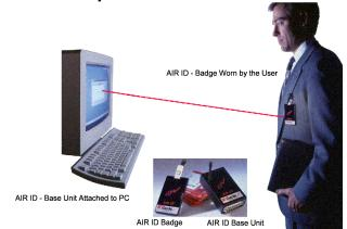
The main components of the AIR ID system are the Base Unit and Badge. The Base Unit is attached to the serial port using the cable and adapter. The badge may be clipped to the user's belt, jacket, collar, inside front pocket, or worn around the neck.
