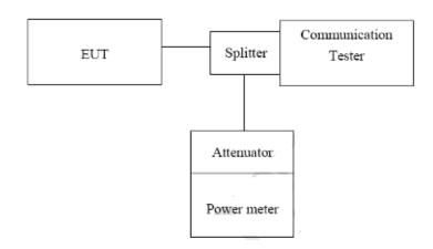
Measurement Setup for testing on Antenna connector.
