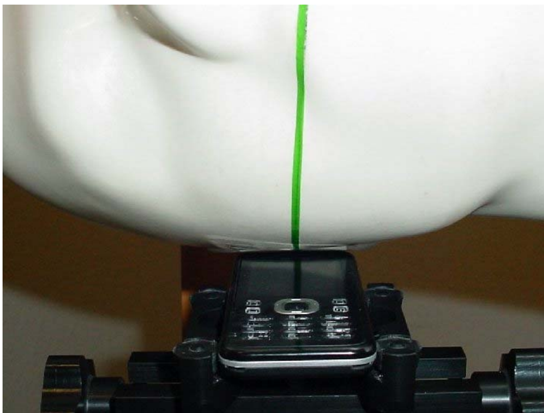
Photo 18: Test position right hand tilted 15°
