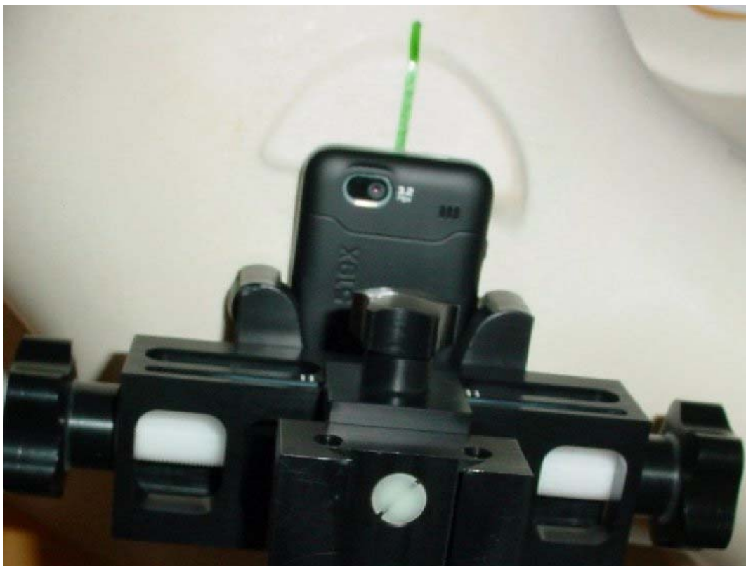
Photo 12: Test position left hand tilted 15°
