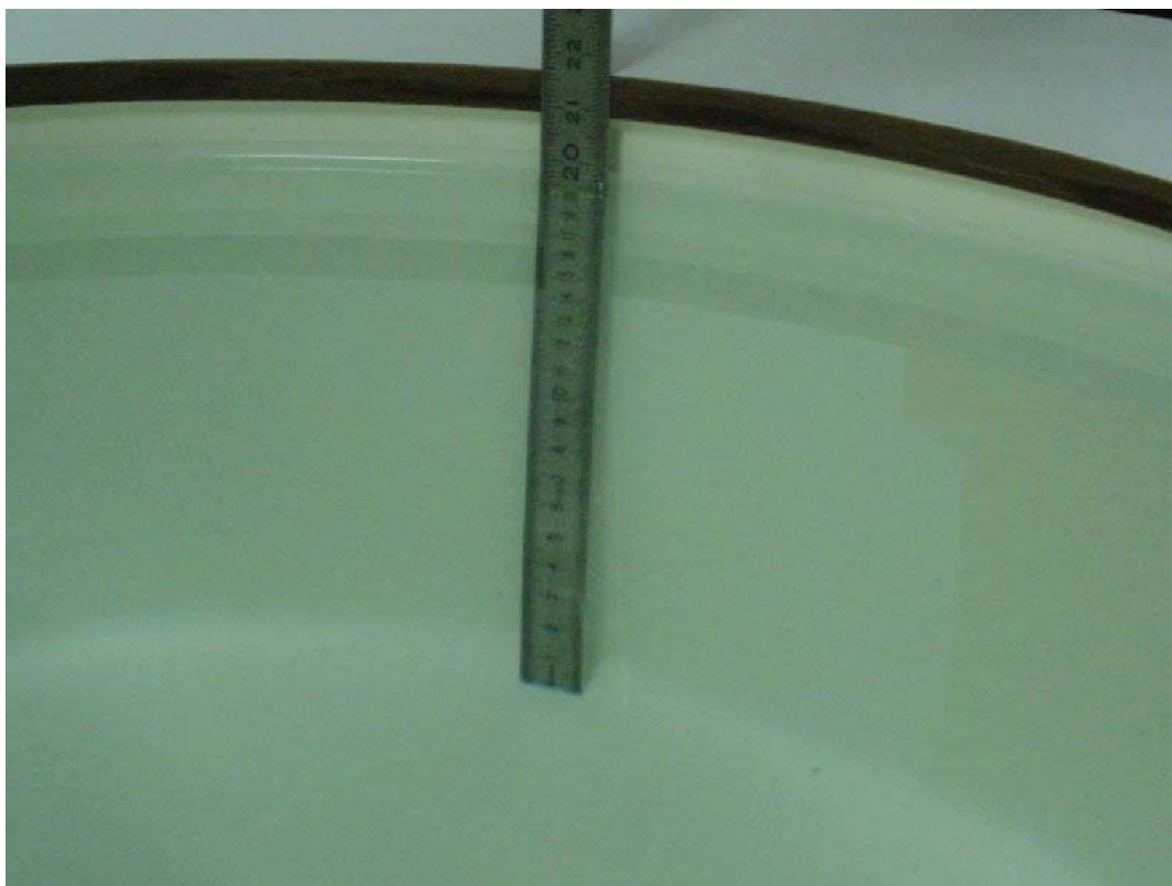
Photo 26: Liquid depth 1900 MHz body simulating liquid
