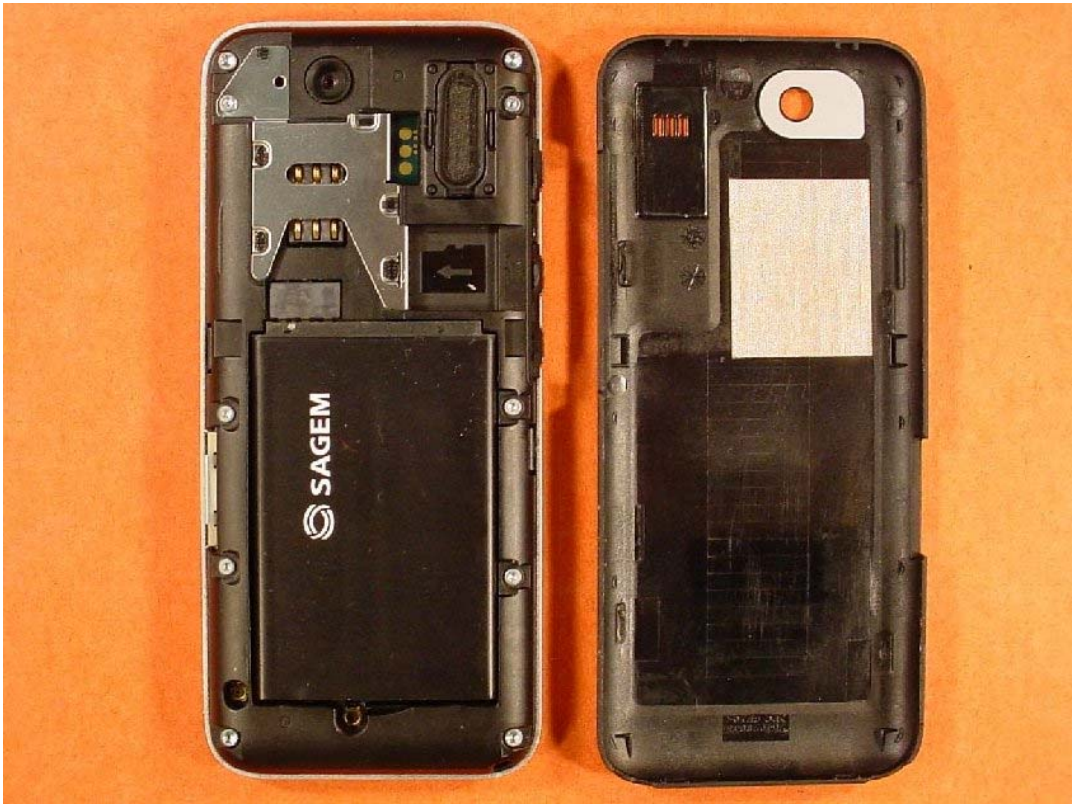
Photo 6: DUT - rear view (open) without battery
