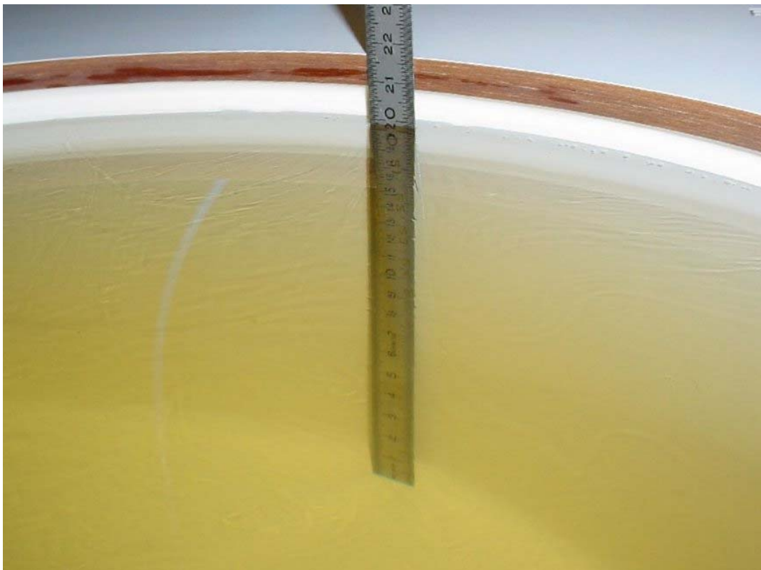
Photo 24: Liquid depth 850 MHz body simulating liquid
