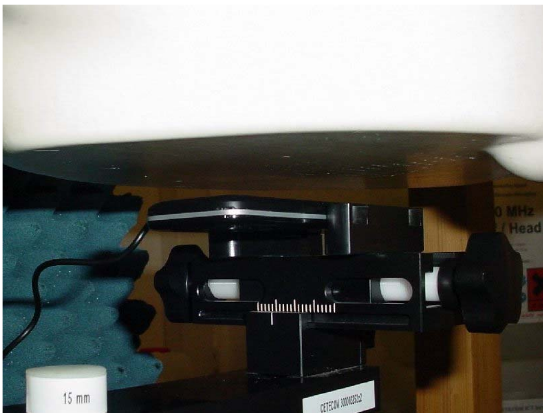
Photo 22: Test position body worn rear side with 15 mm distance
