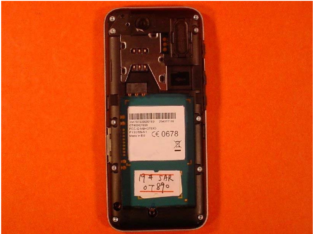
Photo 6: DUT - rear view (open) without battery
