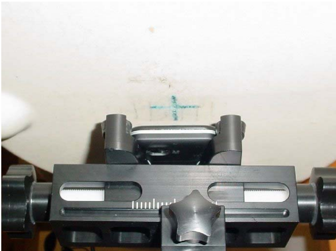
Photo 20: Test position body worn front side with 15 mm distance
