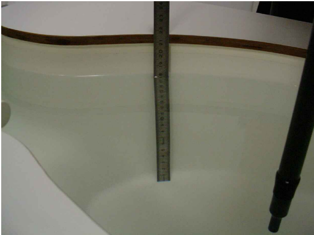
Photo 28: Liquid depth 1900 MHz body simulating liquid
