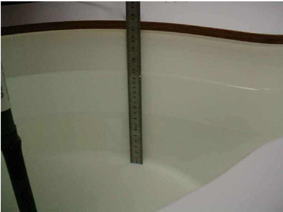
Liquid depth 1900 MHz body simulating liquid
