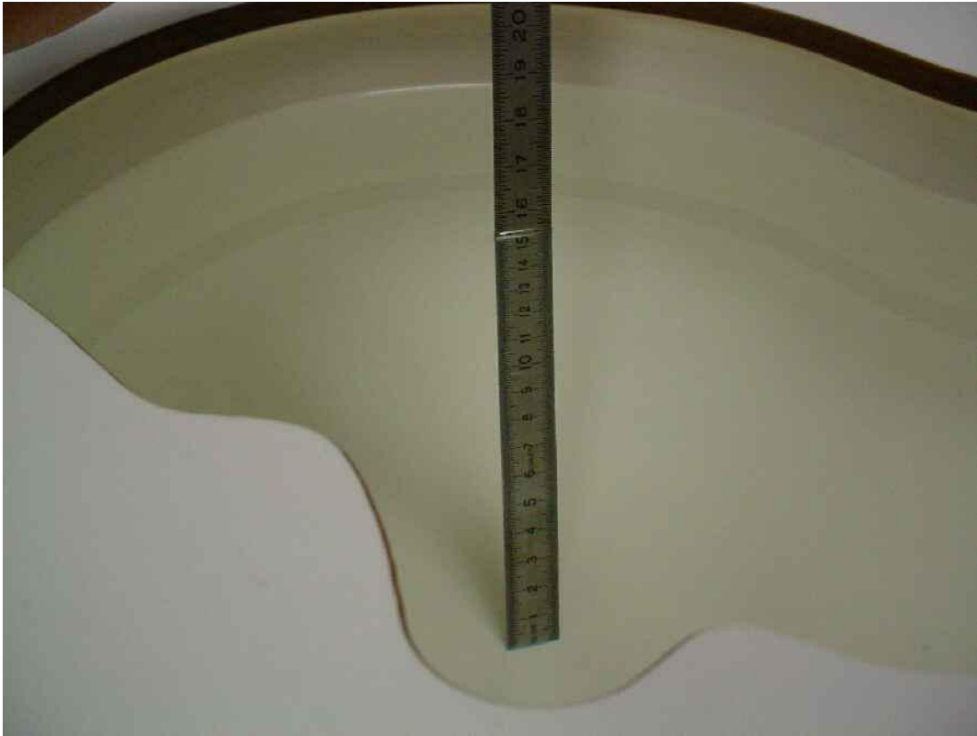
Liquid depth 1900 MHz head simulating liquid
