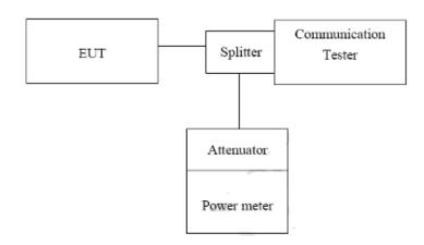
Measurement Setup for testing on Antenna connector.
