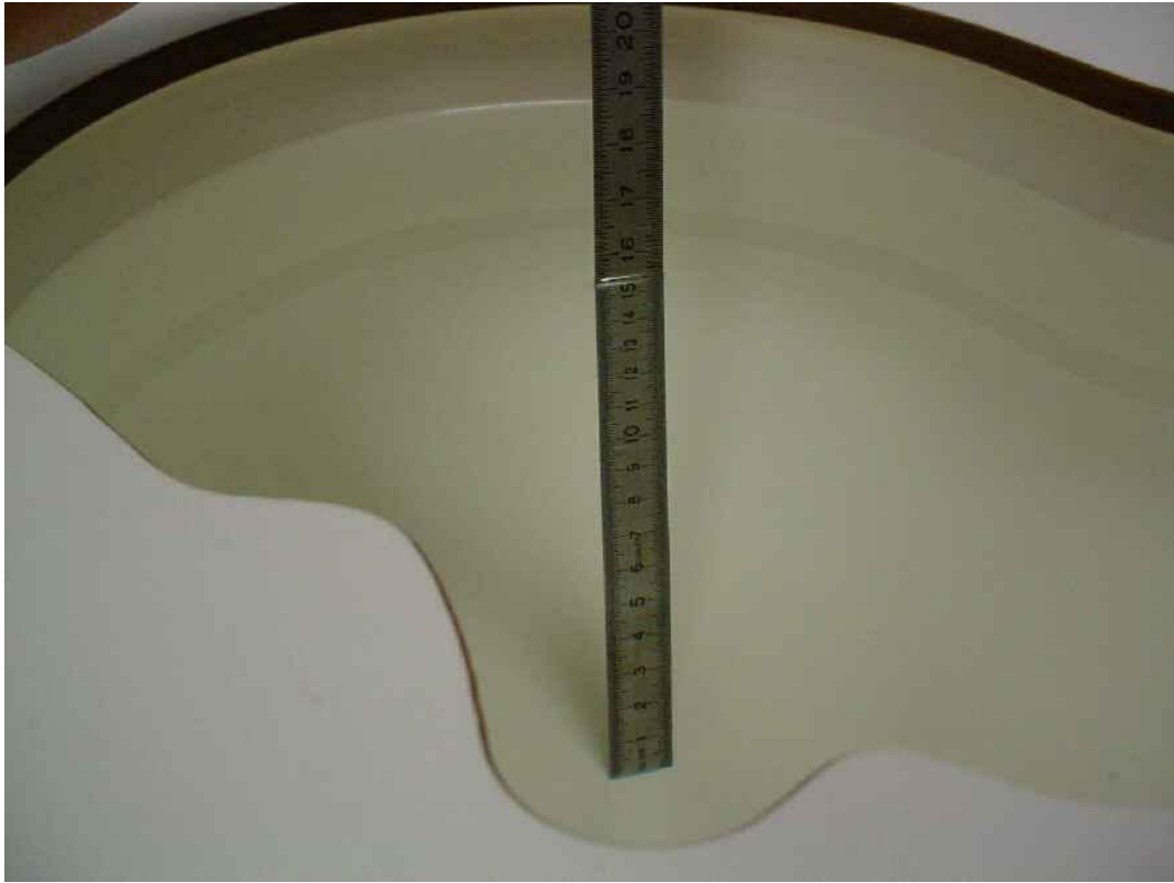
Photo 26: Liquid depth 1900 MHz body simulating liquid
