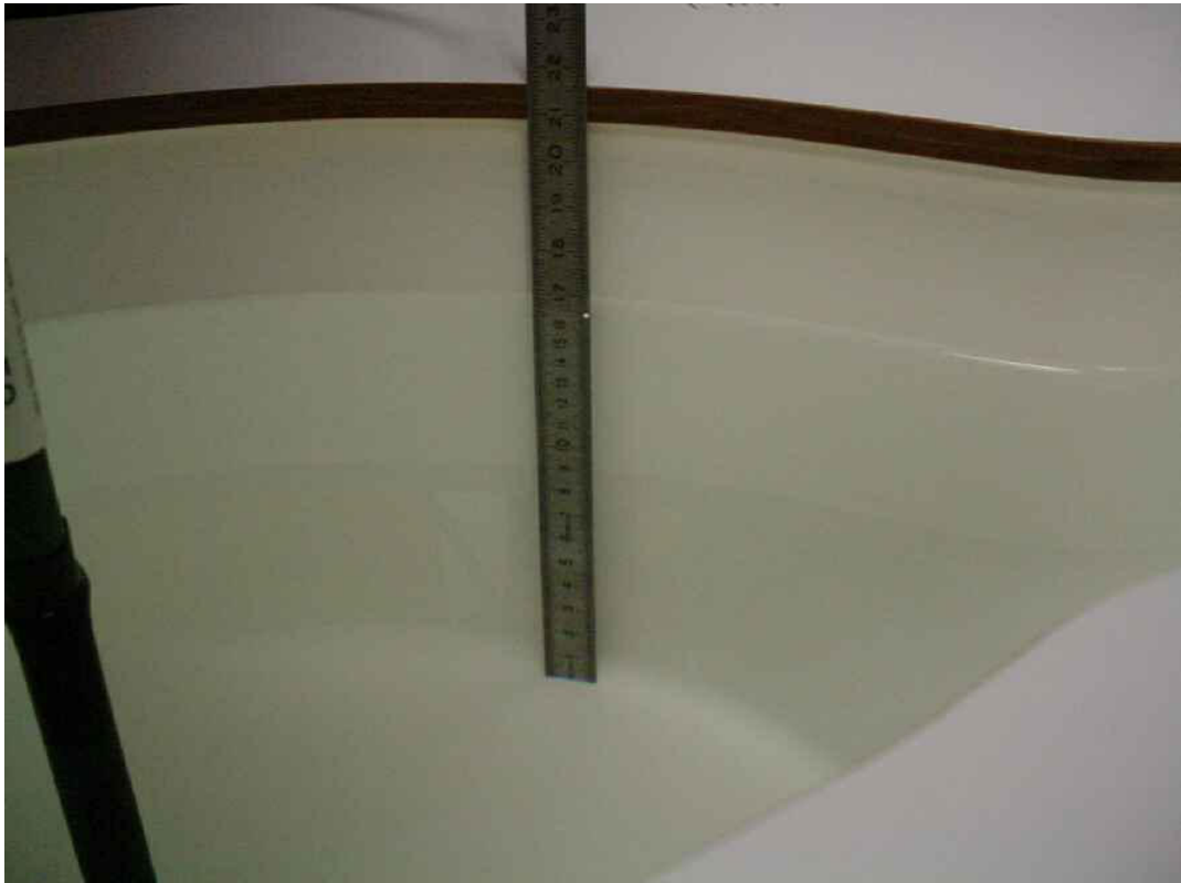
Photo 26: Liquid depth 1900 MHz body simulating liquid
