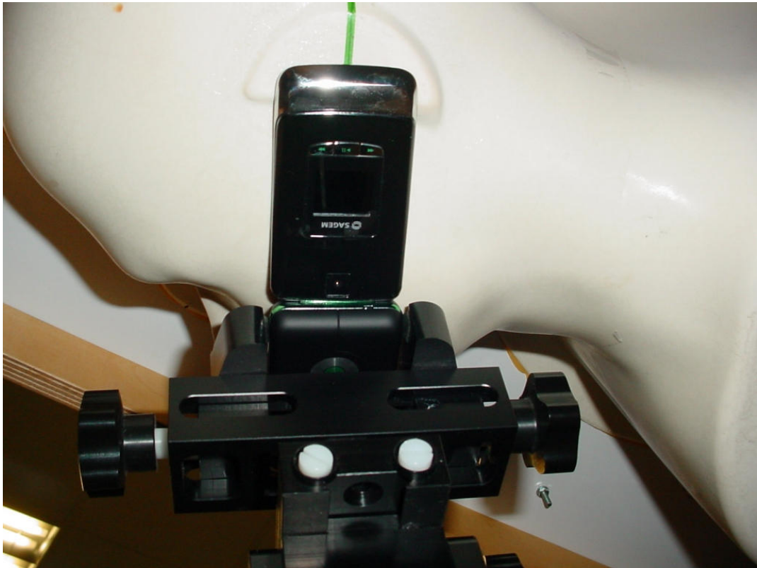
Photo 14: Test position left hand tilted 15°
