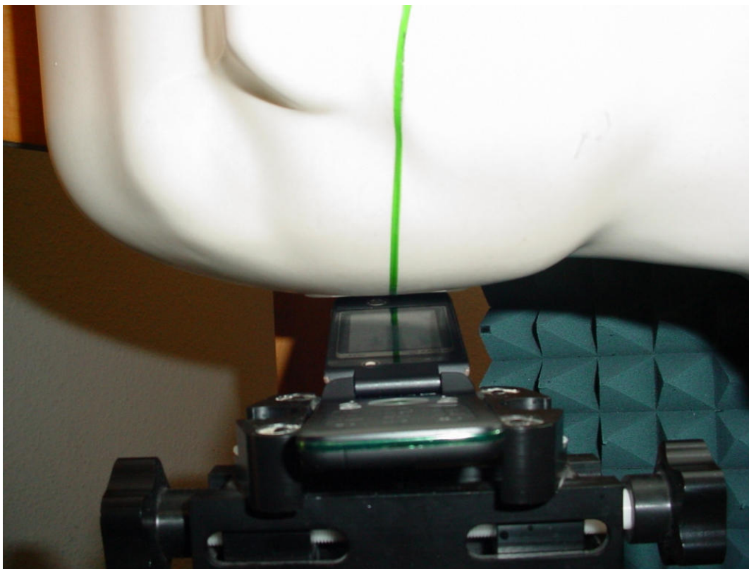
Photo 20: Test position right hand tilted 15°
