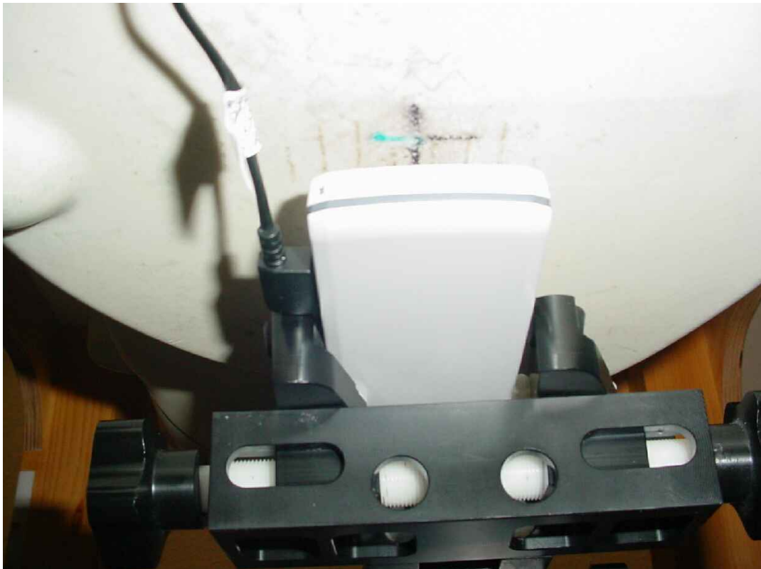
Photo 23: Test position body worn front side (distance 15 mm) with Remote control (189345890) + headset (189346219)
