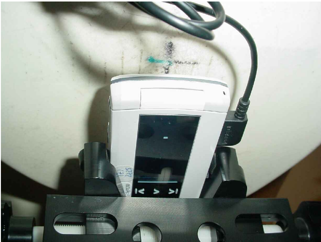
Photo 27: Test position body worn rear side (distance 15 mm) with Stereo headset EMB-SGC712AYBA (189515468)
