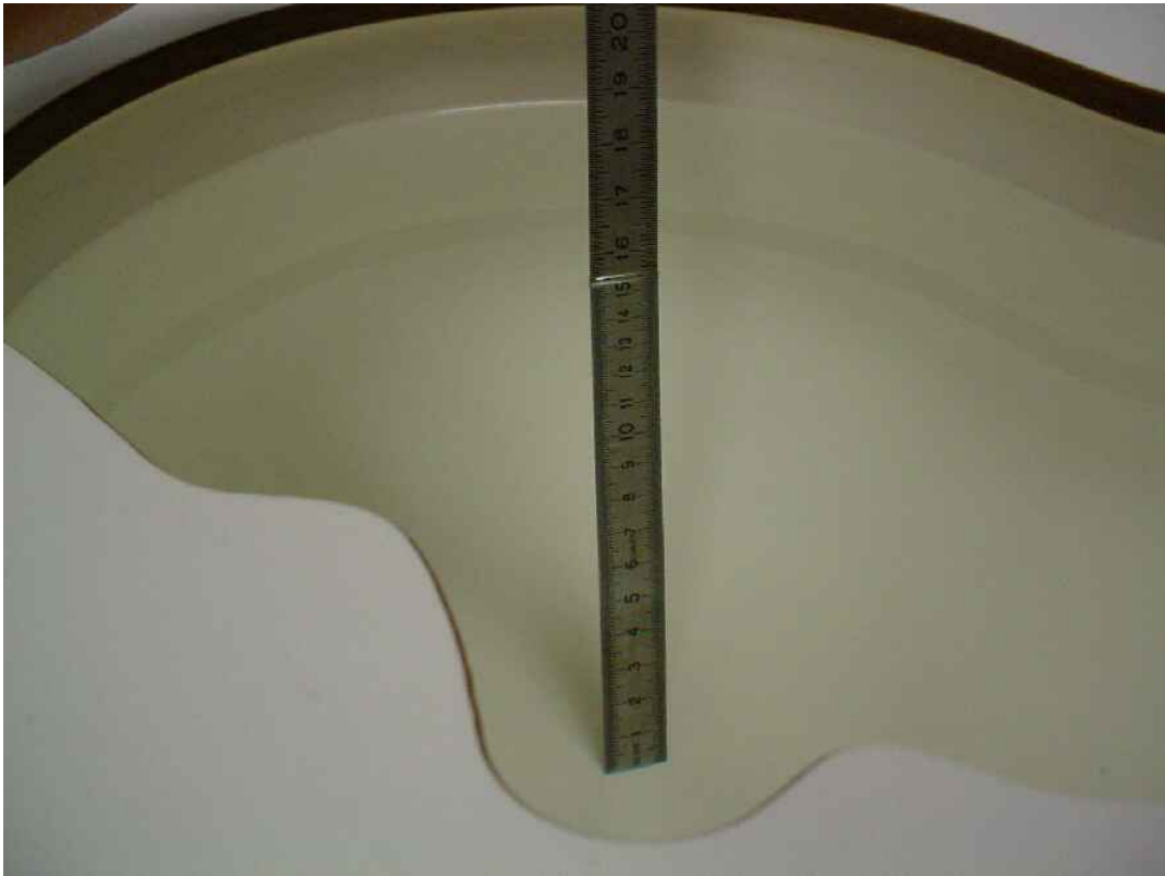
Photo 32: Liquid depth 1900 MHz body simulating liquid
