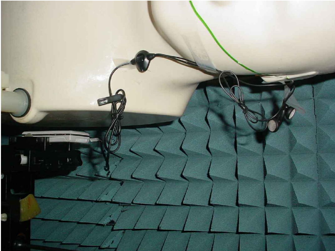
Photo 28: Test position body worn rear side (distance 15 mm) with Stereo headset EMB-SGC712AYBA (189515468)
