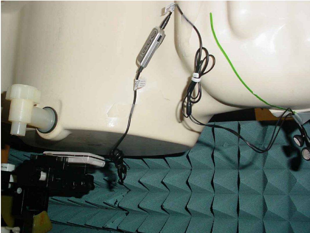
Photo 26: Test position body worn rear side (distance 15 mm) with Remote control (189345890) + headset (189346219)
