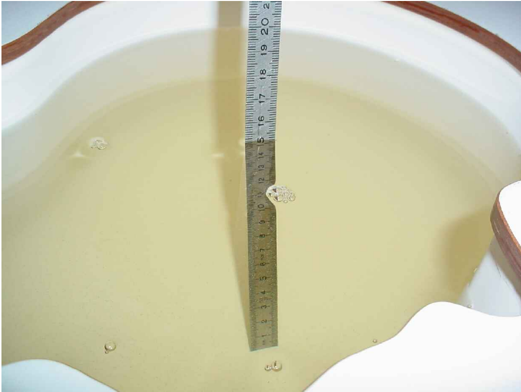
Photo 30: Liquid depth 850 MHz body simulating liquid
