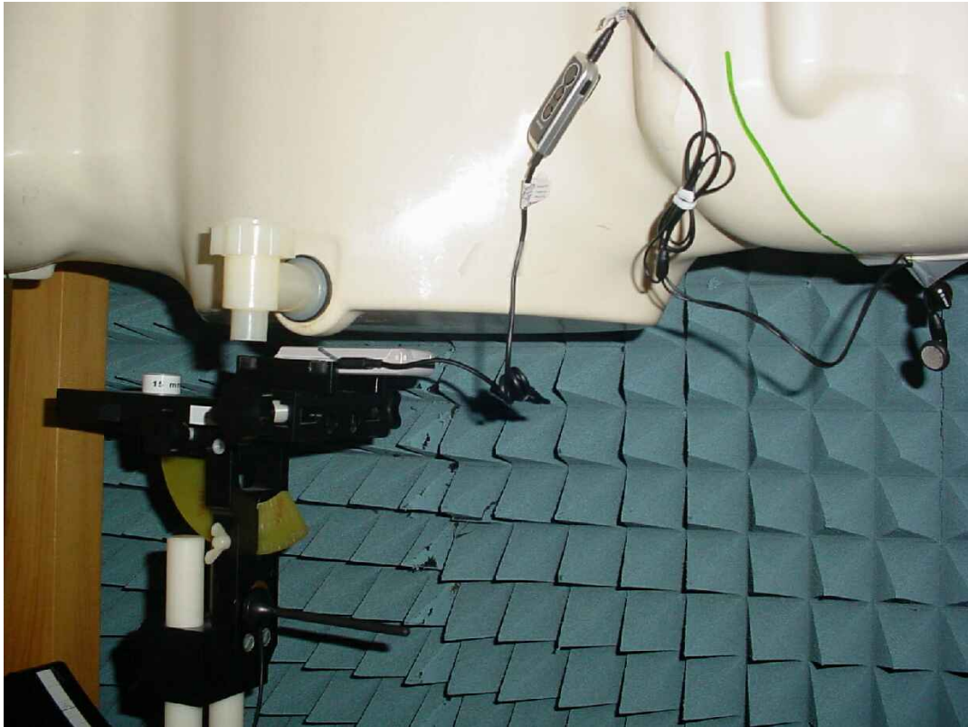
Photo 24: Test position body worn front side (distance 15 mm) with Remote control (189345890) + headset (189346219)
