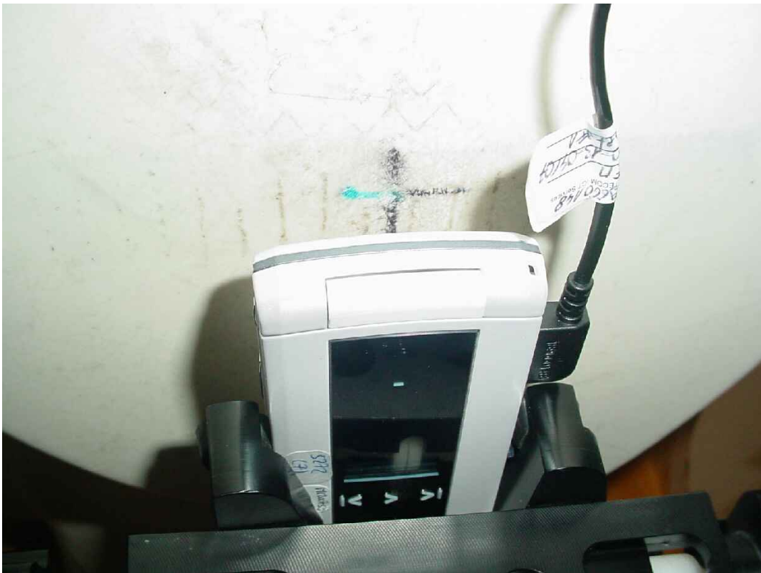
Photo 28: Test position body worn rear side (distance 15 mm) with Stereo headset EMB-SGC712AYBA (189515468)
