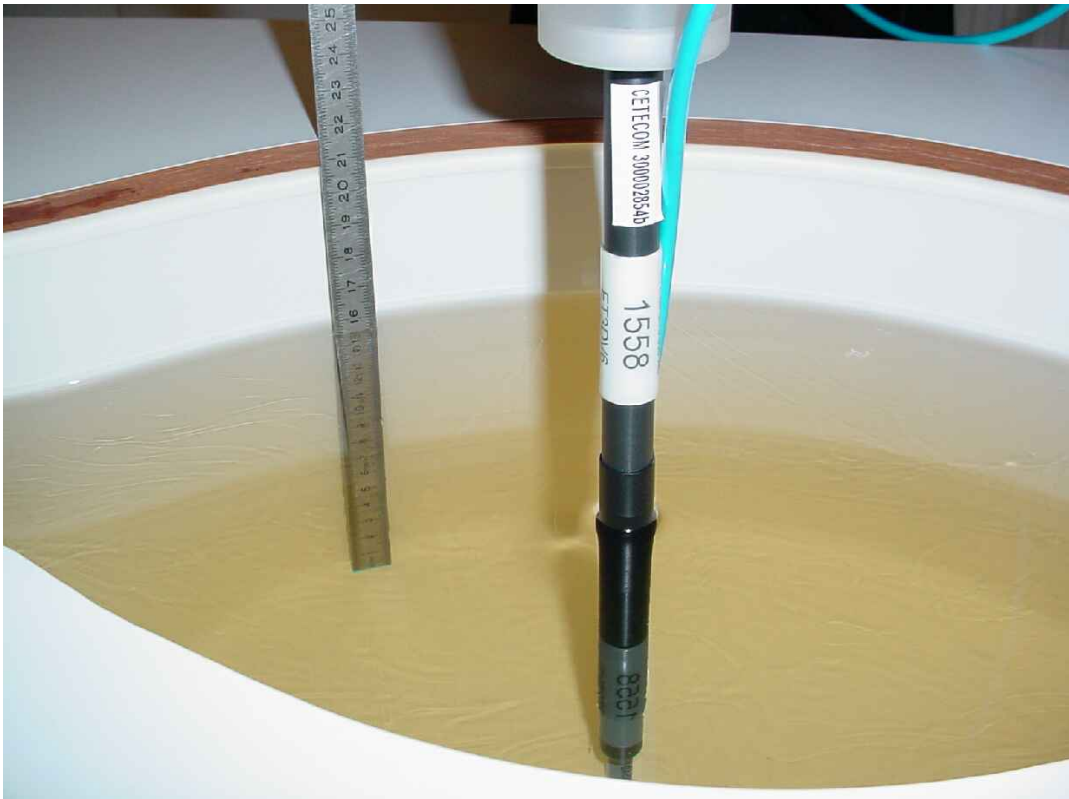
Photo 30: Liquid depth 850 MHz body simulating liquid
