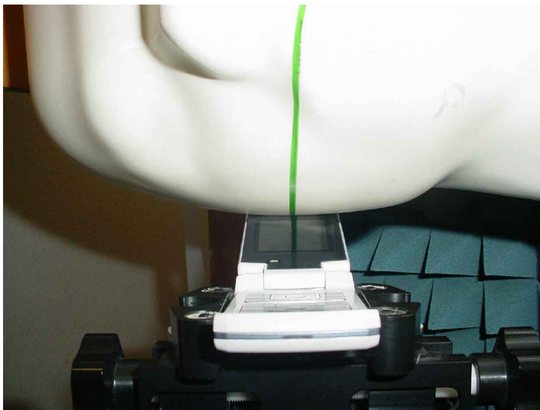
Photo 20: Test position right hand tilted 15°
