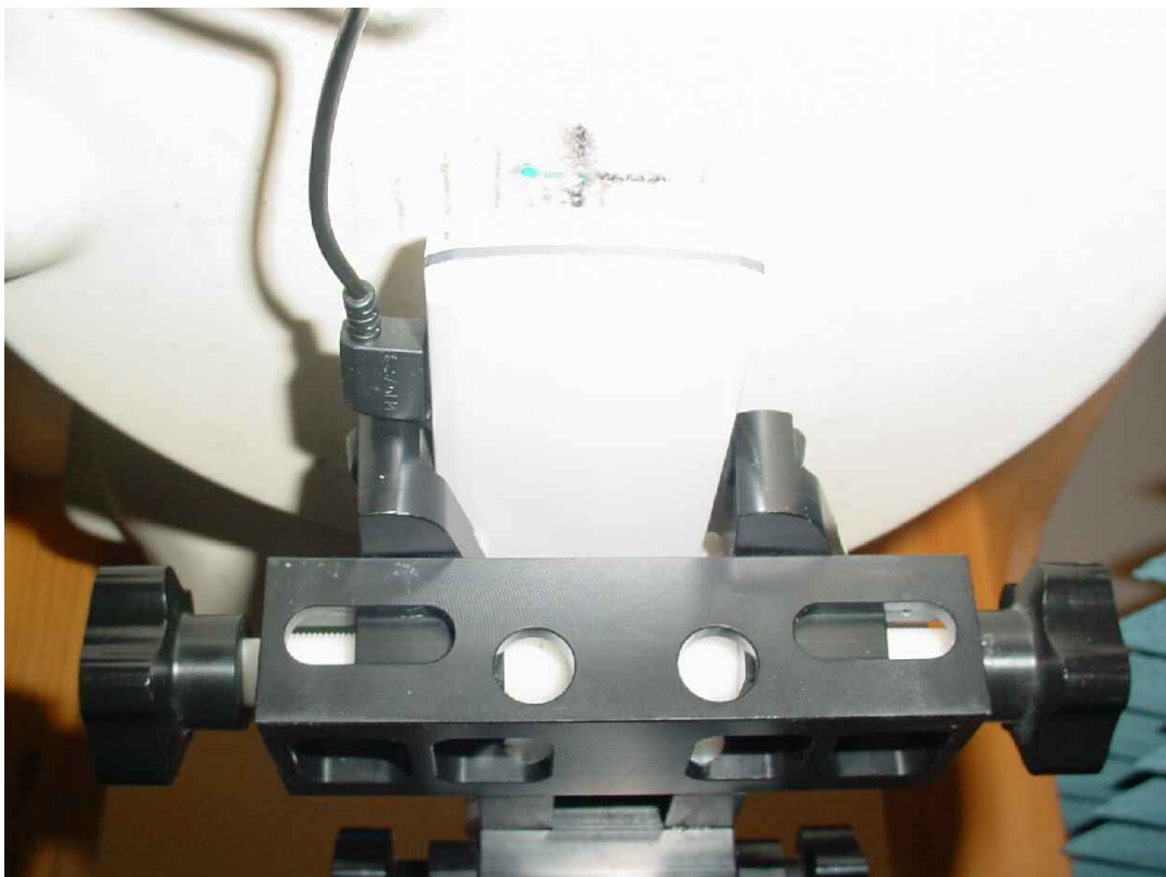
Photo 25: Test position body worn rear side (distance 15 mm) with Remote control (189345890) + headset (189346219)
