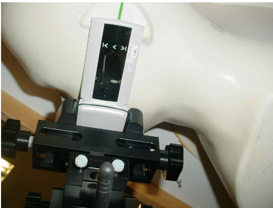
Photo 14: Test position left hand tilted 15°
