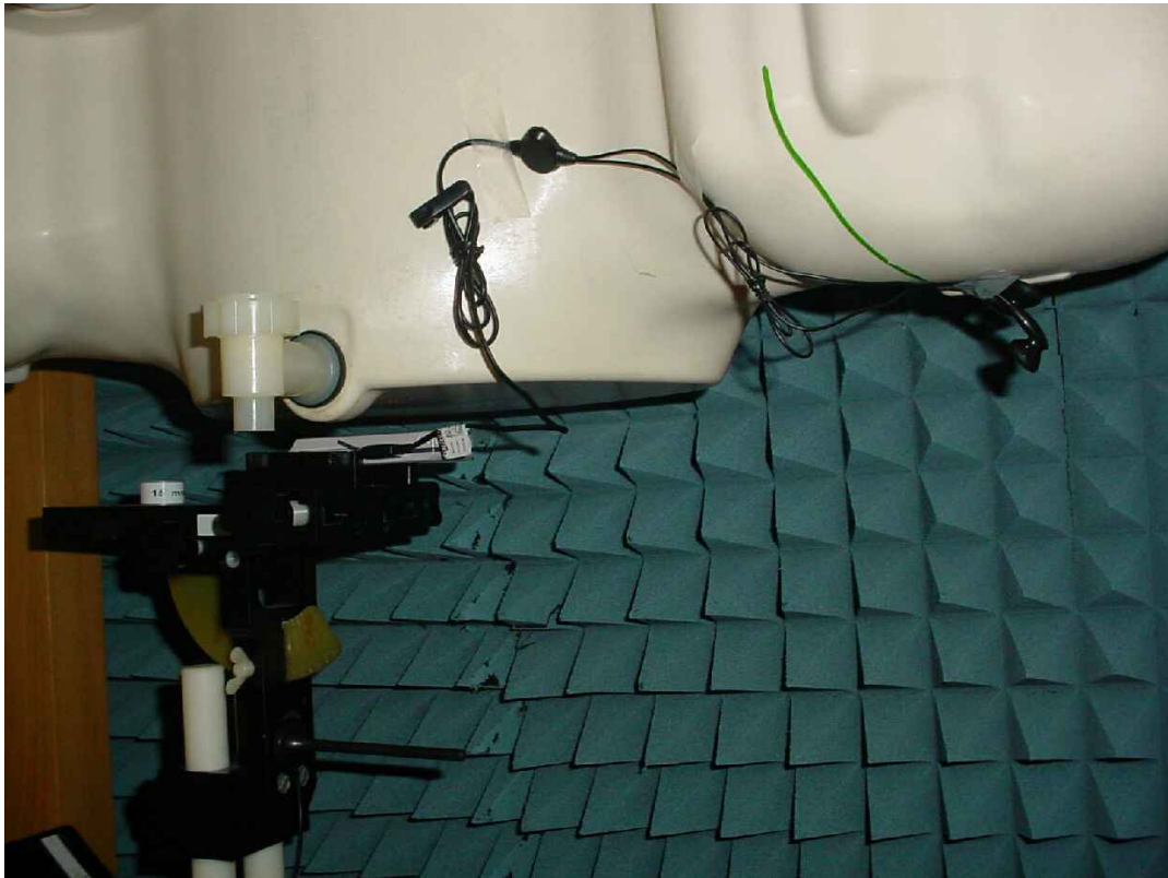
Photo 22: Test position body worn front side (distance 15 mm) with stereo headset EMB-SGC712AYBA (189515468)
