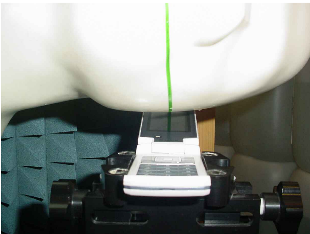
Photo 14: Test position left hand tilted 15°
