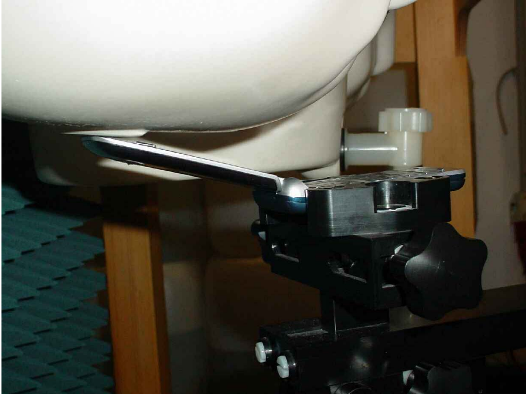
Photo 21: Test position body worn front side (distance 15 mm) with stereo headset EMB-SGC712AYBB (189660148)
