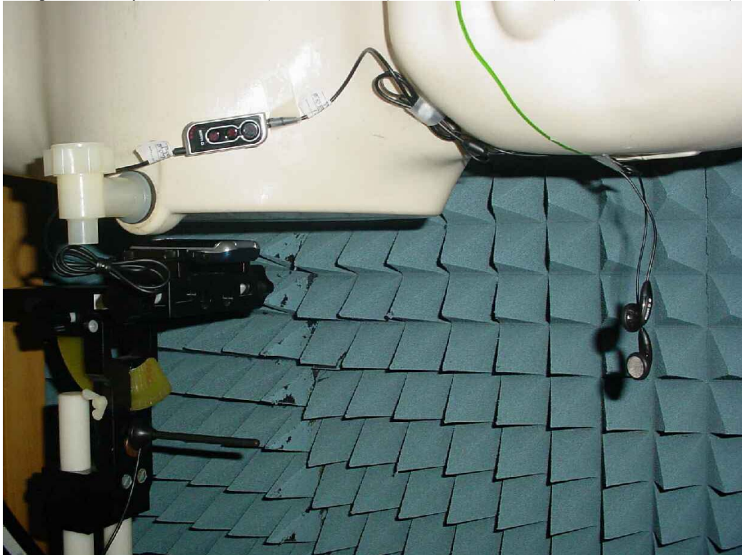
Photo 26: Test position body worn front side (distance 15 mm) with remote control (189345890) + headset (189346219)
