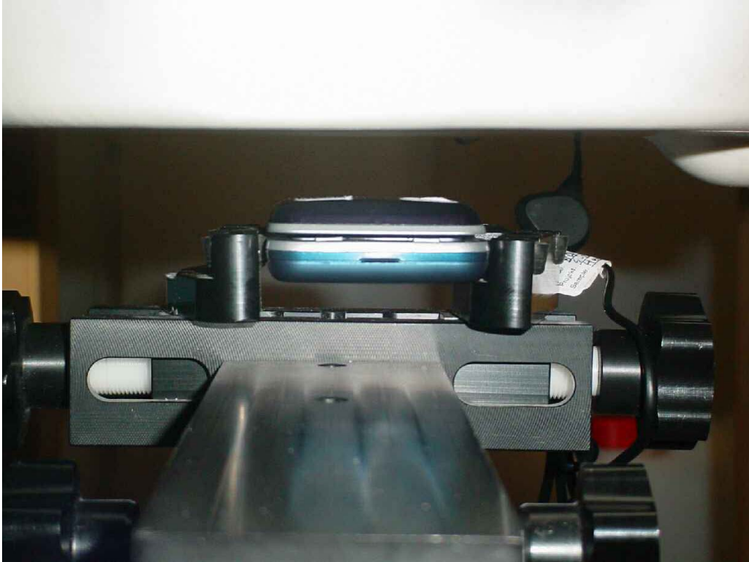
Photo 23: Test position body worn front side (distance 15 mm) with stereo headset EMB- SGC712AYBB (189660148)
