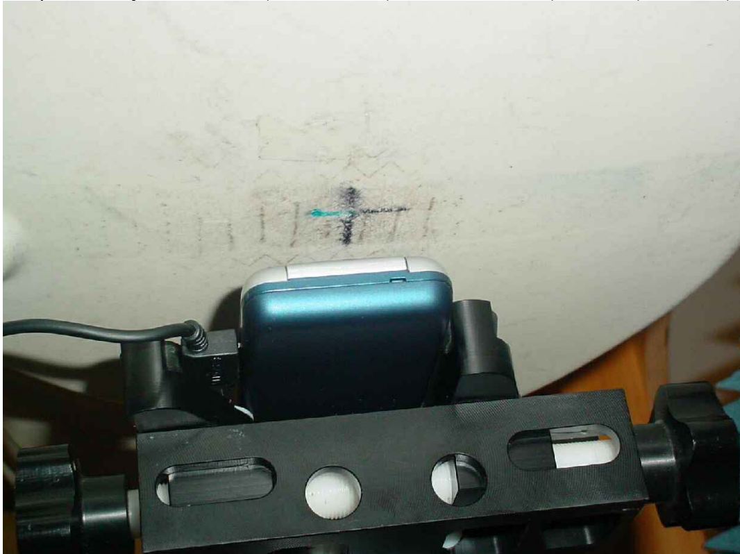
Photo 27: Test position body worn front side (distance 15 mm) with remote control (189345890) + headset (189346219)
