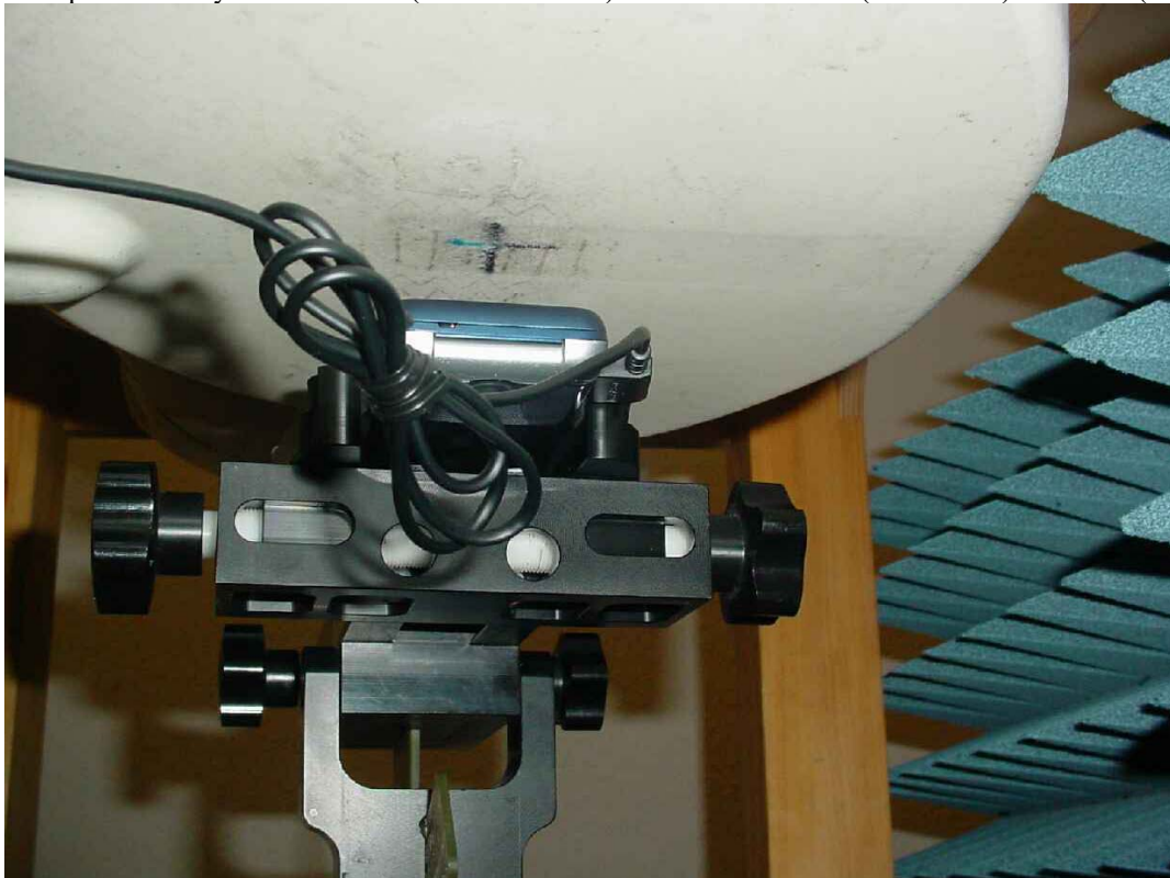
Photo 29: Test position body worn rear side (distance 15 mm) with remote control (189345890) + headset (189346219)
