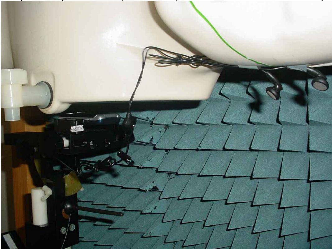
Photo 21: Test position body worn front side (distance 15 mm) with stereo headset EMB-SGC712AYBB (189660148)
