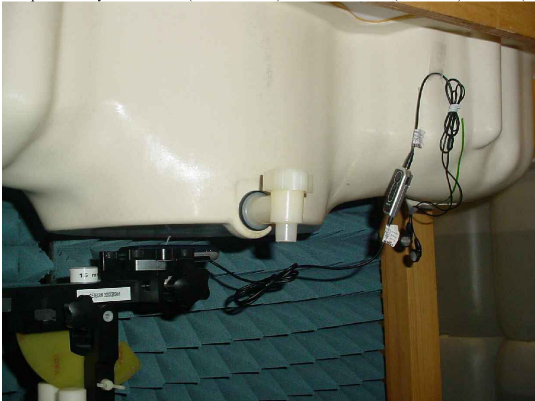
Photo 29: Test position body worn rear side (distance 15 mm) with remote control (189345890) + headset (189346219)
