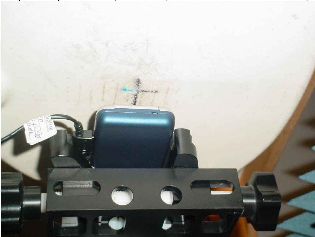
Photo 23: Test position body worn front side (distance 15 mm) with stereo headset EMB- SGC712AYBB (189660148)
