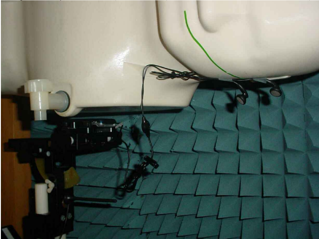
Photo 25: Test position body worn rear side (distance 15 mm) with stereo headset EMB- SGC712AYBB (189660148)
