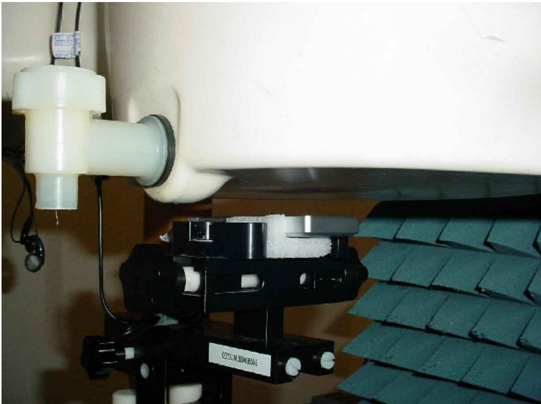
Photo 18: Test position body worn front side (15 mm distance)
