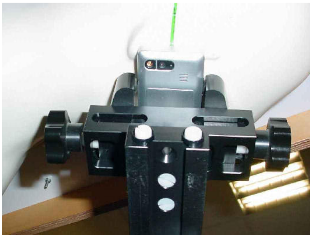
Photo 16: Test position right hand tilted 15°
