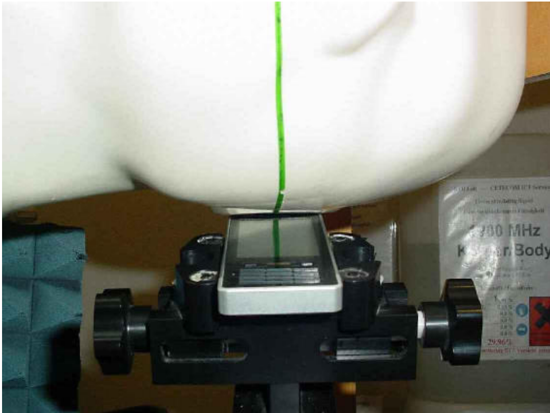
Photo 12: Test position left hand tilted 15°
