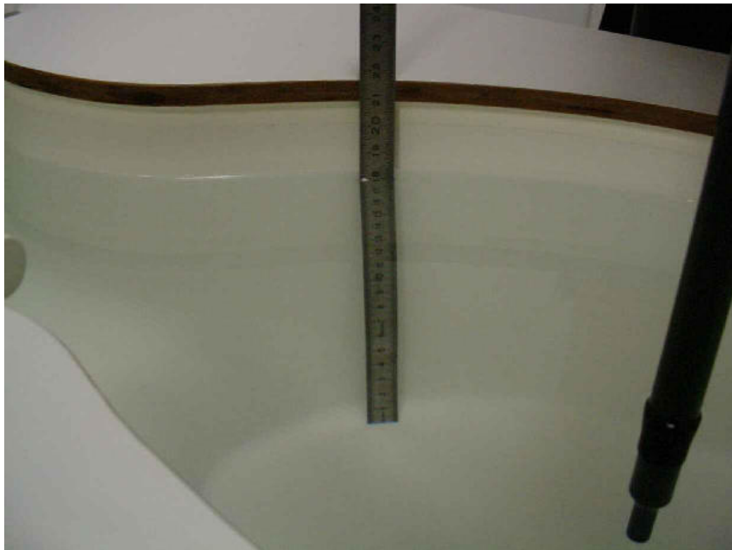
Photo 27: Liquid depth 2450 MHz body simulating liquid
