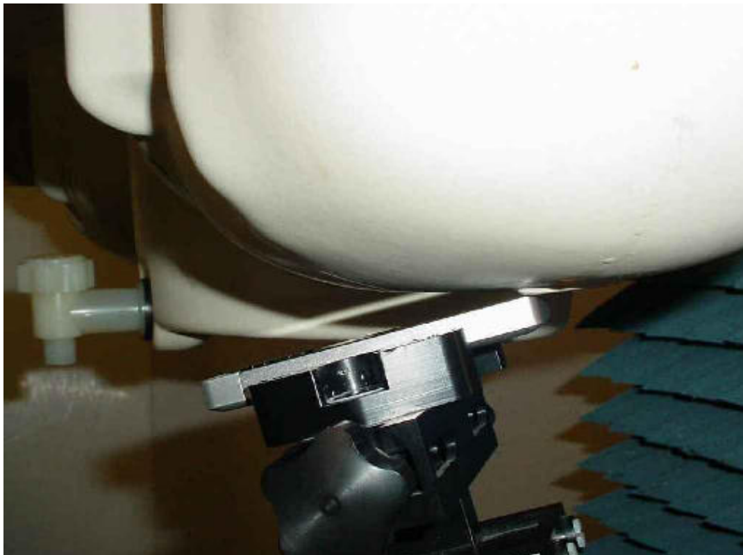
Photo 12: Test position left hand tilted 15°
