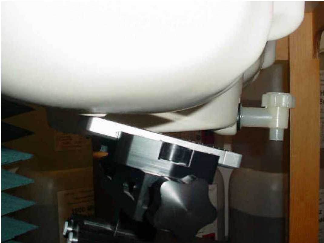
Photo 18: Test position body worn front side (15 mm distance)
