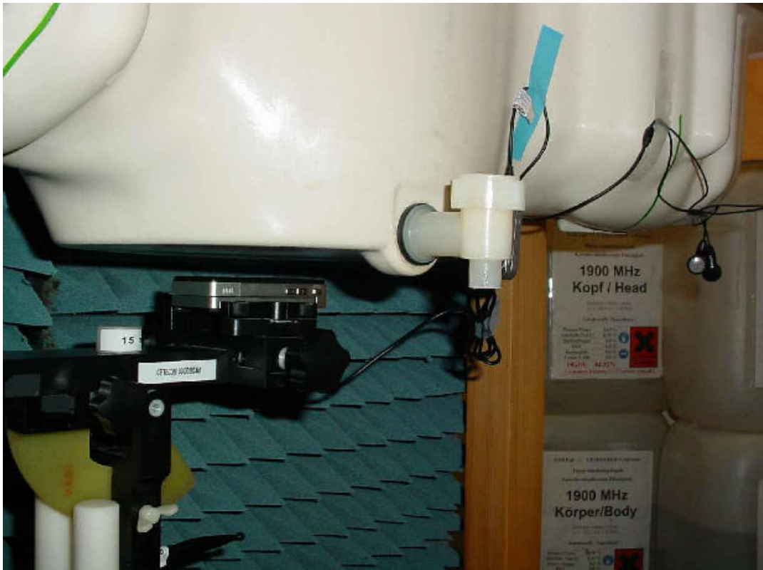
Photo 26: Test position body worn rear side turned over (15 mm distance)
