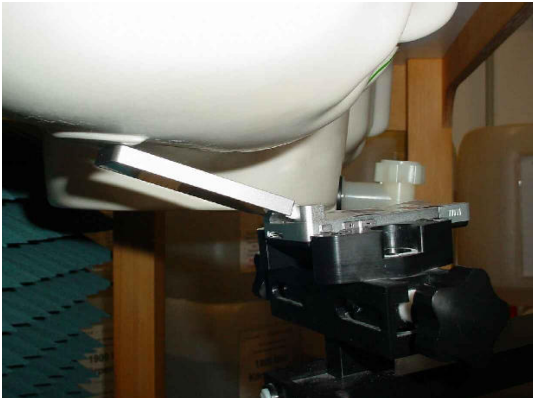
Photo 20: Test position right hand tilted 15°
