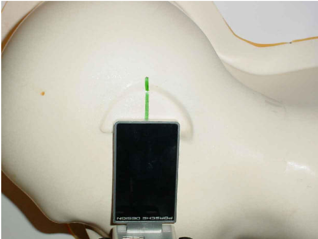
Photo 14: Test position left hand tilted 15°
