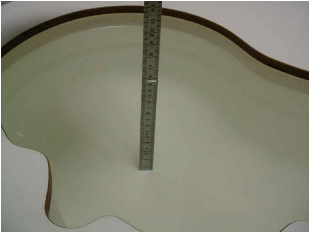
Photo 31: Liquid depth 1900 MHz body simulating liquid
