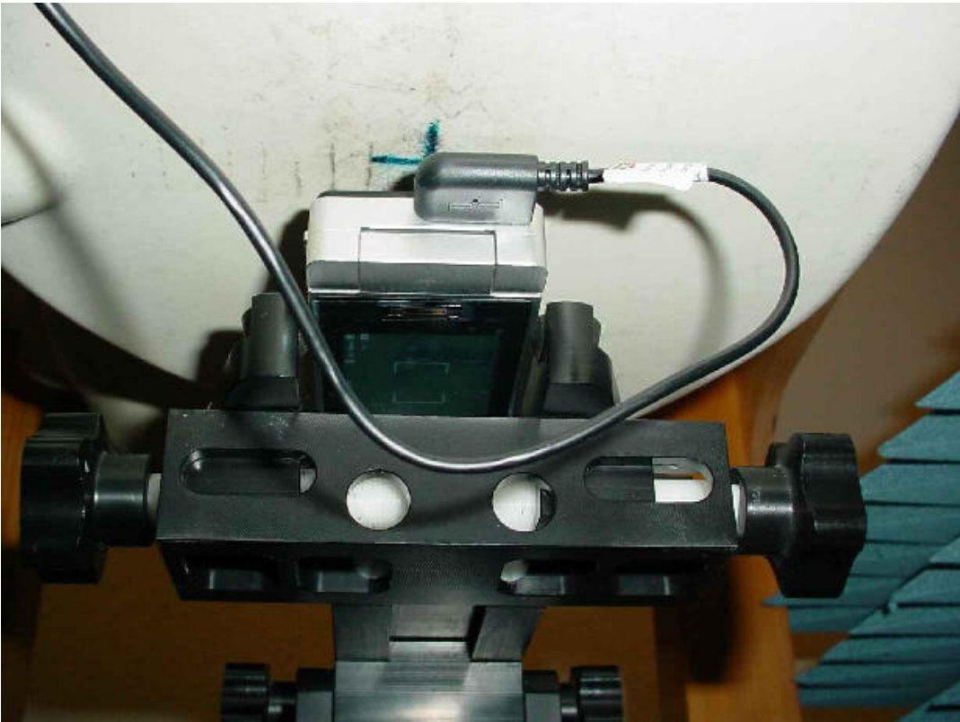
Photo 27: Test position body worn rear side turned over (15 mm distance)
