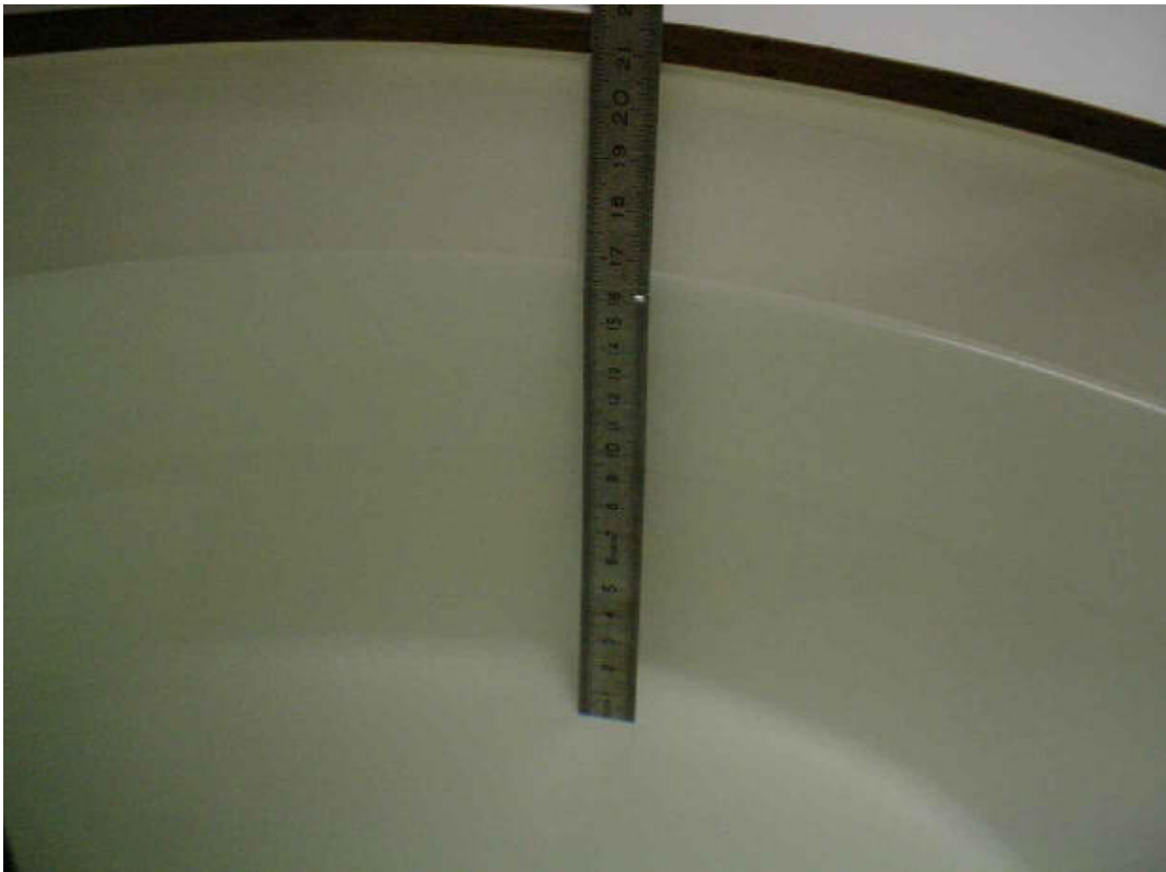
Photo 31: Liquid depth 1900 MHz body simulating liquid
