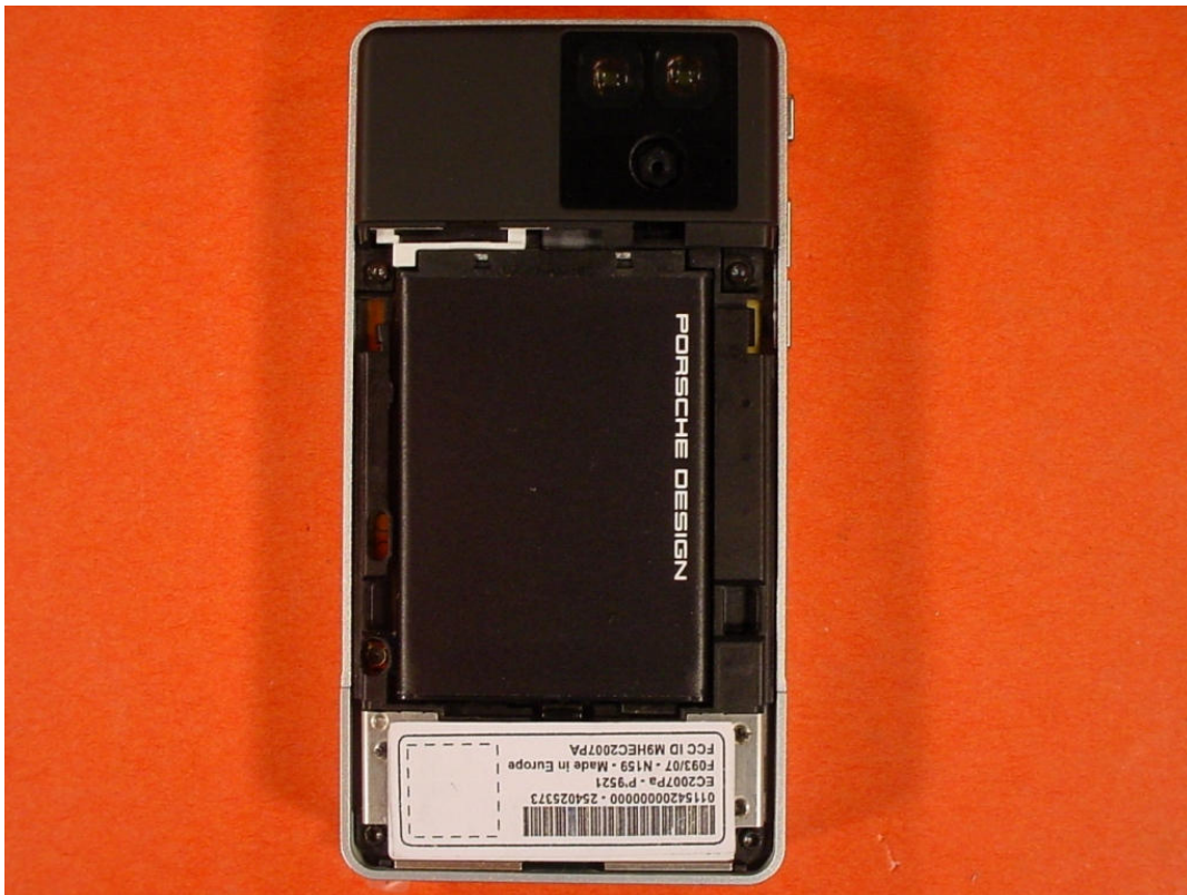
Photo 8: DUT - rear view (open) without battery
