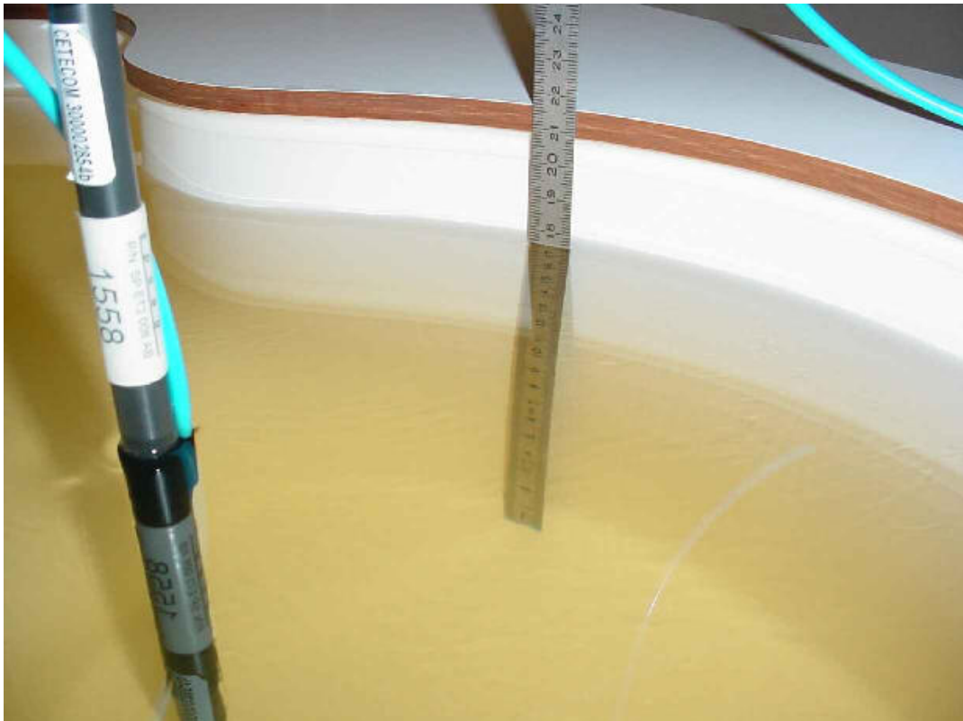
Photo 29: Liquid depth 850 MHz body simulating liquid
