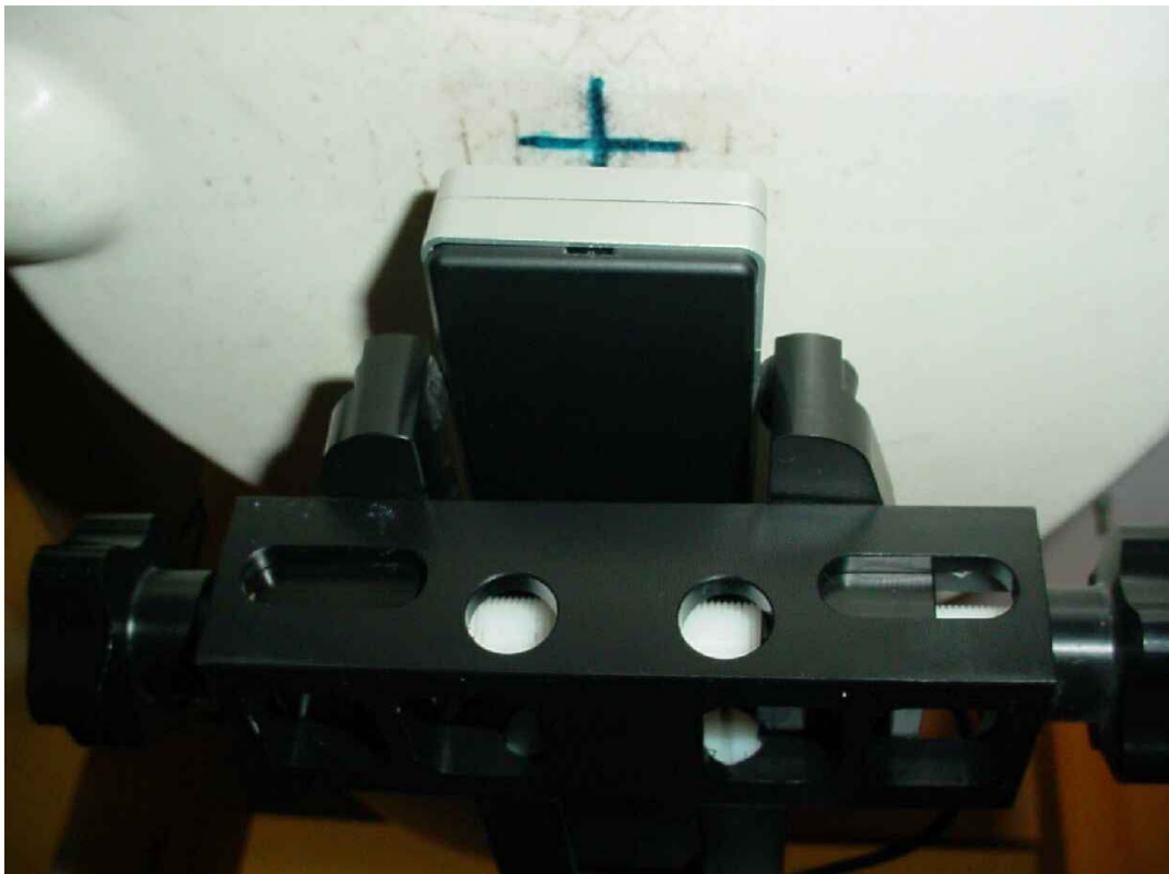
Photo 26: Test position body worn front side (distance 15 mm)
