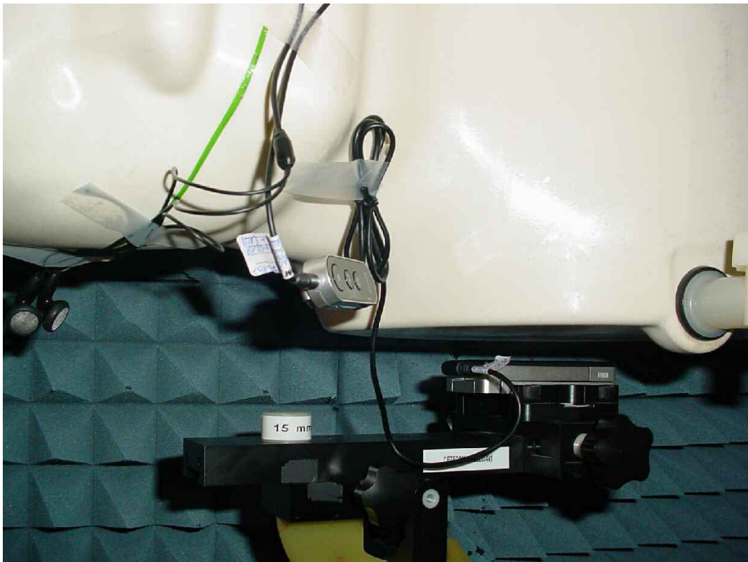
Photo 28: Test position body worn rear side (distance 15 mm)
