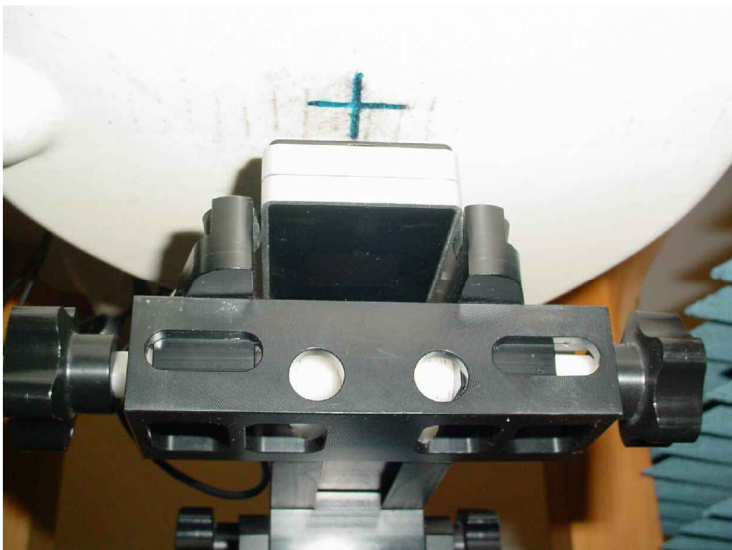
Photo 28: Test position body worn rear side (distance 15 mm)
