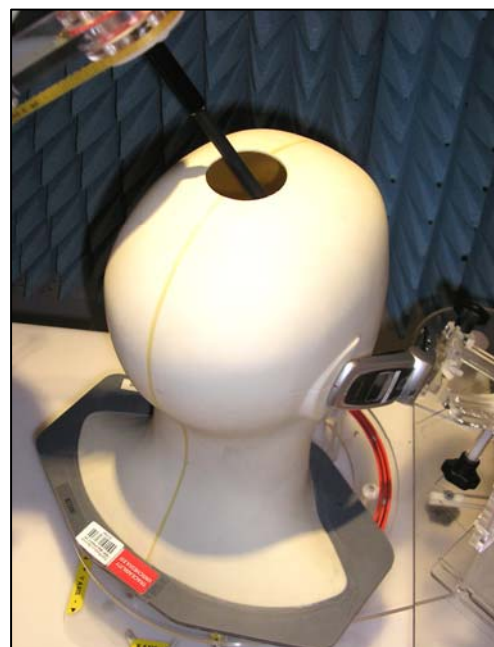
Figure 30: Positional Photograph of the Sagem DC2006a Handset in RH 15° Position (SAR Head Test)
