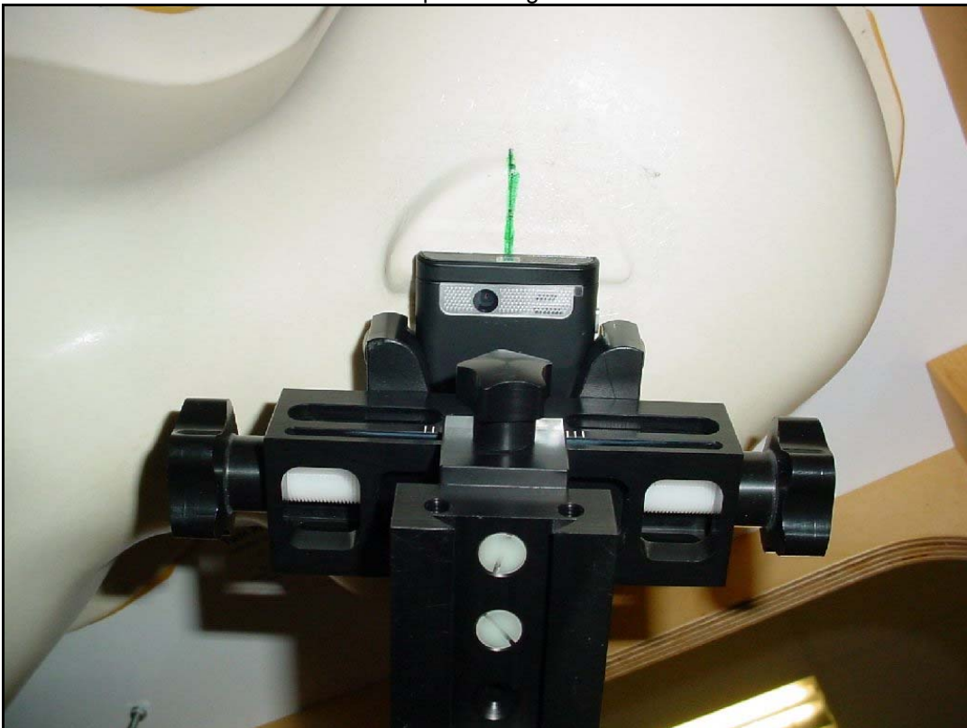
Photo 16: Test position right hand touched
