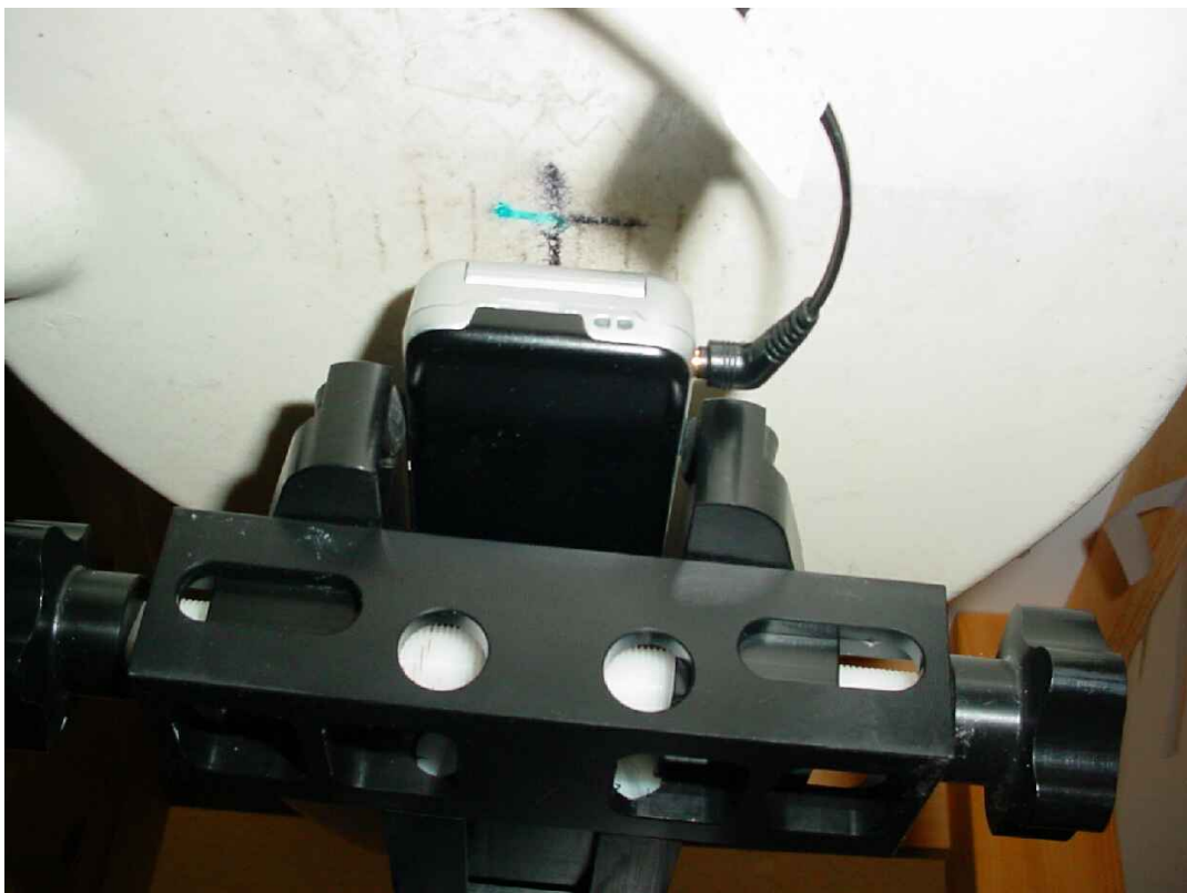
Photo 26: Test position body worn front side (15 mm distance) with stereo headset (189551609)
