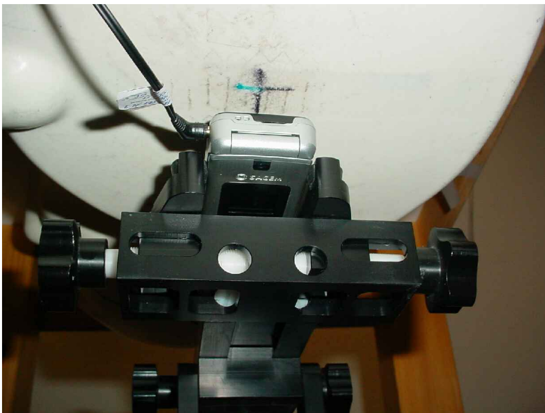
Photo 33: Test position body worn front side (15 mm distance) with mono headset (189507169)
