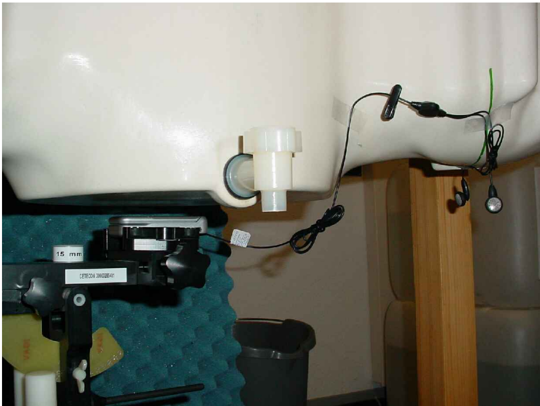
Photo 27: Test position body worn front side (15 mm distance) with stereo headset (189551609)
