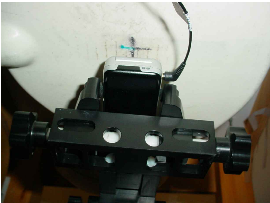
Photo 28: Test position body worn rear side (15 mm distance) with stereo headset (189551609)
