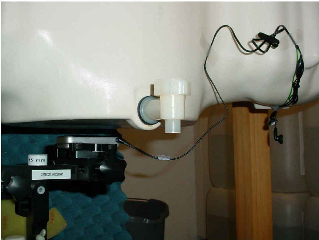
Photo 31: Test position body worn rear side (15 mm distance) with stereo headset (179092963)
