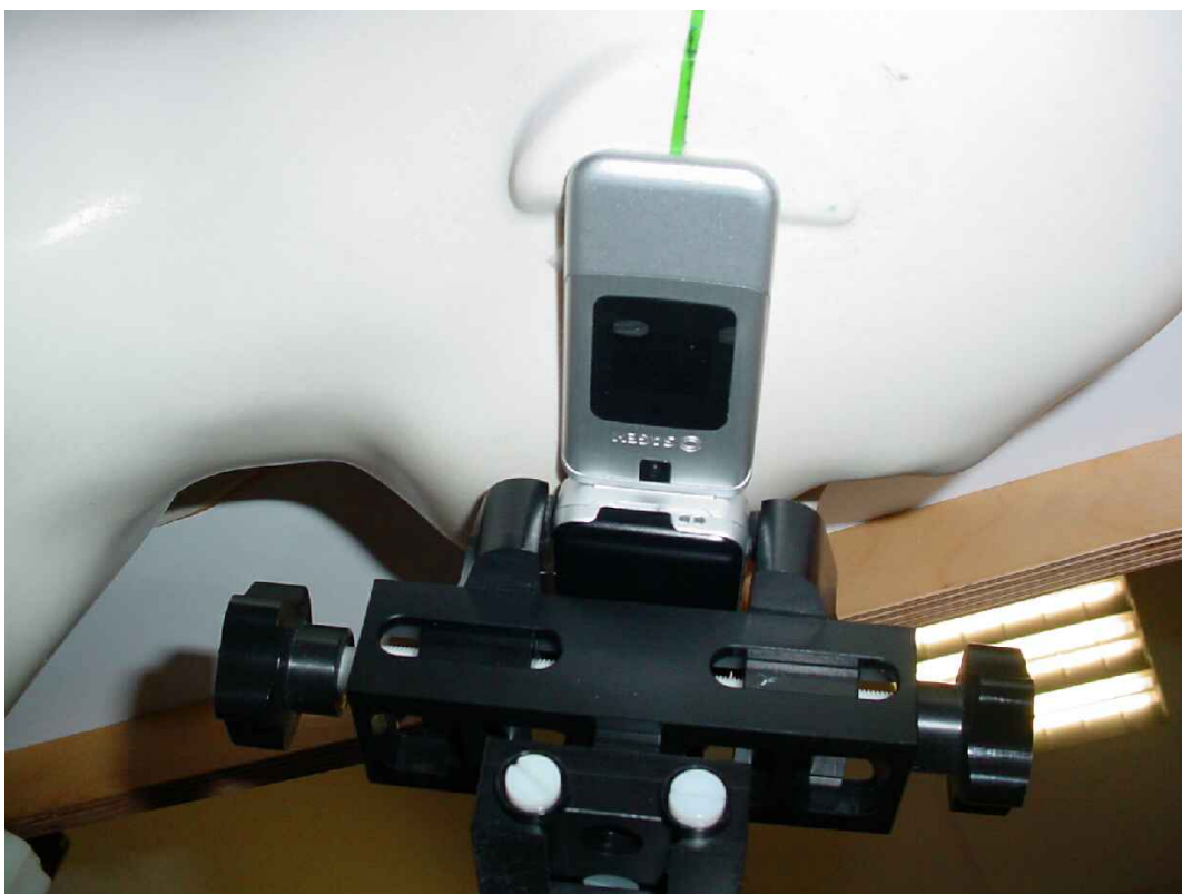
Photo 19: Test position right hand touched
