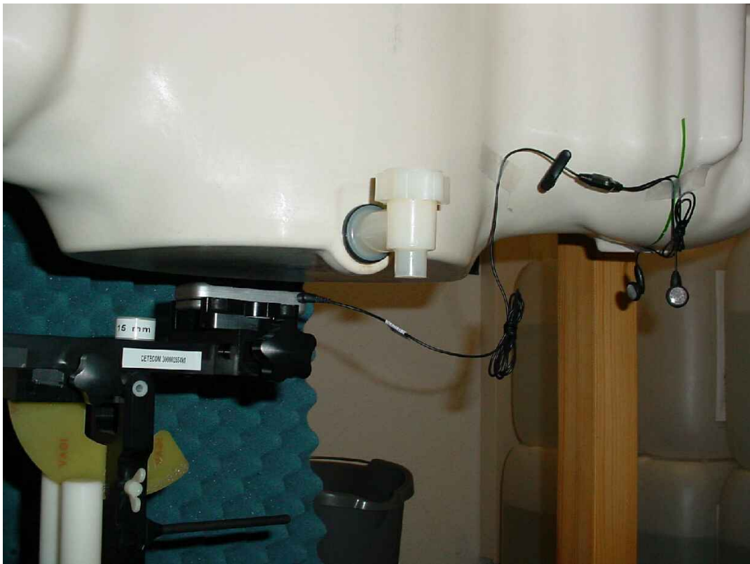
Photo 29: Test position body worn rear side (15 mm distance) with stereo headset (189551609)
