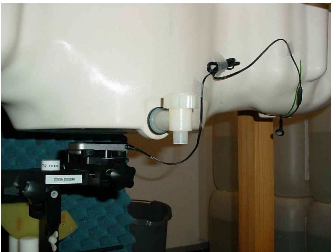
Photo 33: Test position body worn front side (15 mm distance) with mono headset (189507169)
