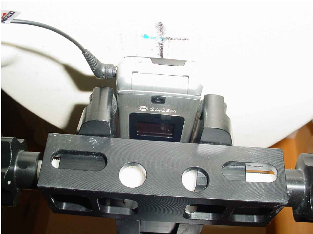
Photo 30: Test position body worn rear side (15 mm distance) with stereo headset (179092963)
