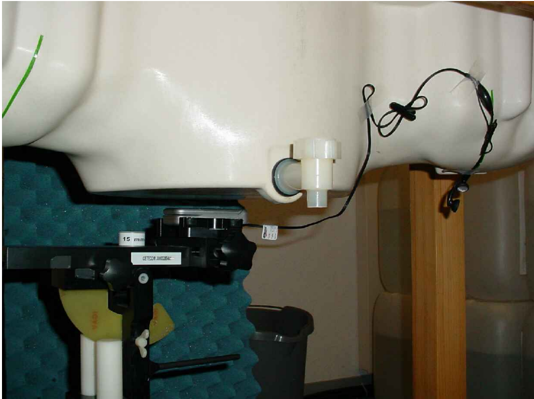
Photo 25: Test position body worn front side (15 mm distance) with stereo headset (179092963)
