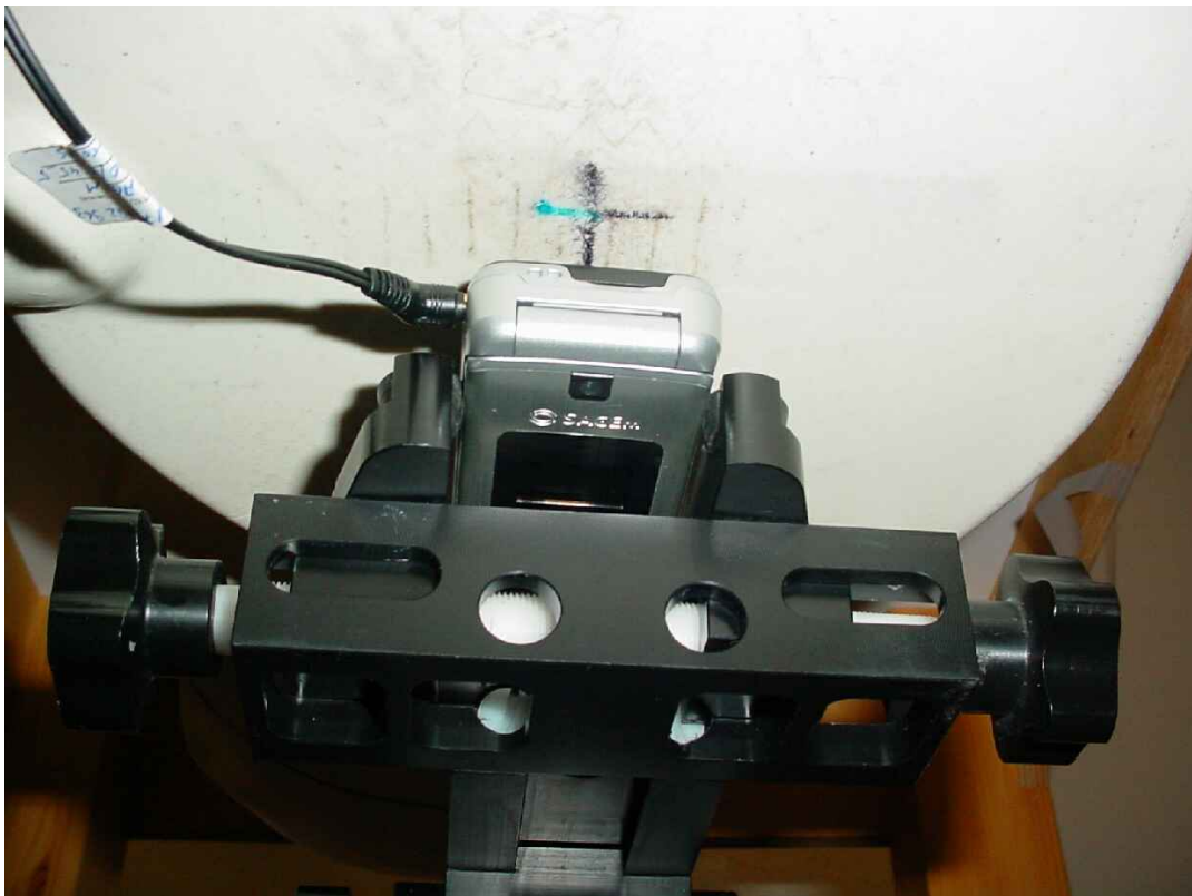
Photo 32: Test position body worn front side (15 mm distance) with mono headset (189507169)
