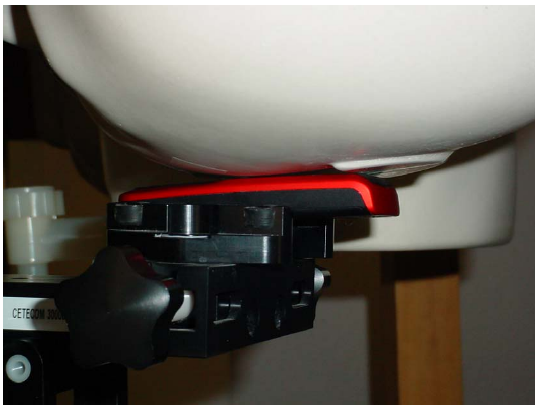
Photo 8: Test position left hand touched
