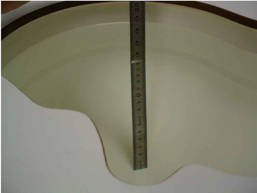
Photo 24: Liquid depth 1900 MHz body simulating liquid
