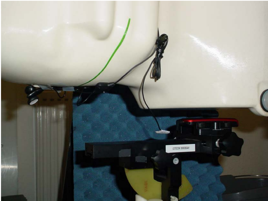
Photo 18: Test position body worn front side (distance 15mm) with stereo headset
