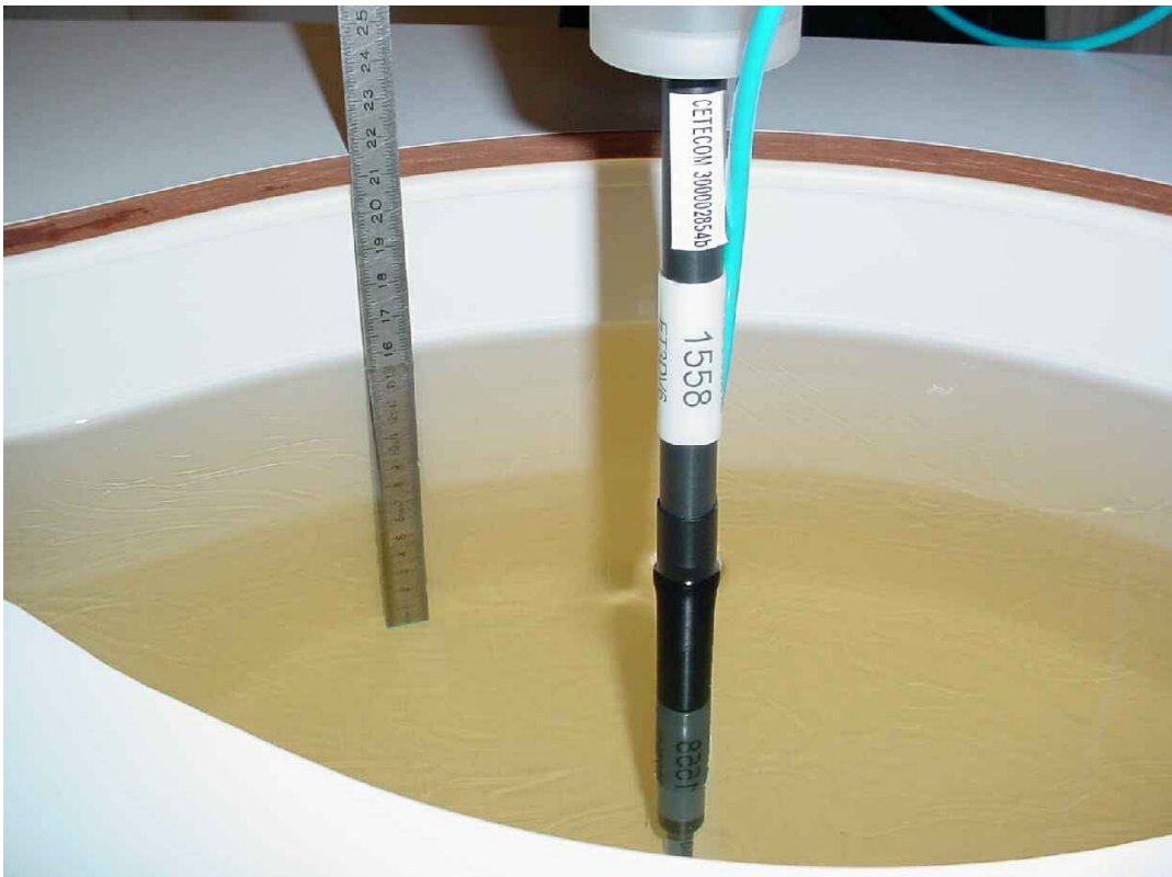
Photo 22: Liquid depth 850 MHz body simulating liquid
