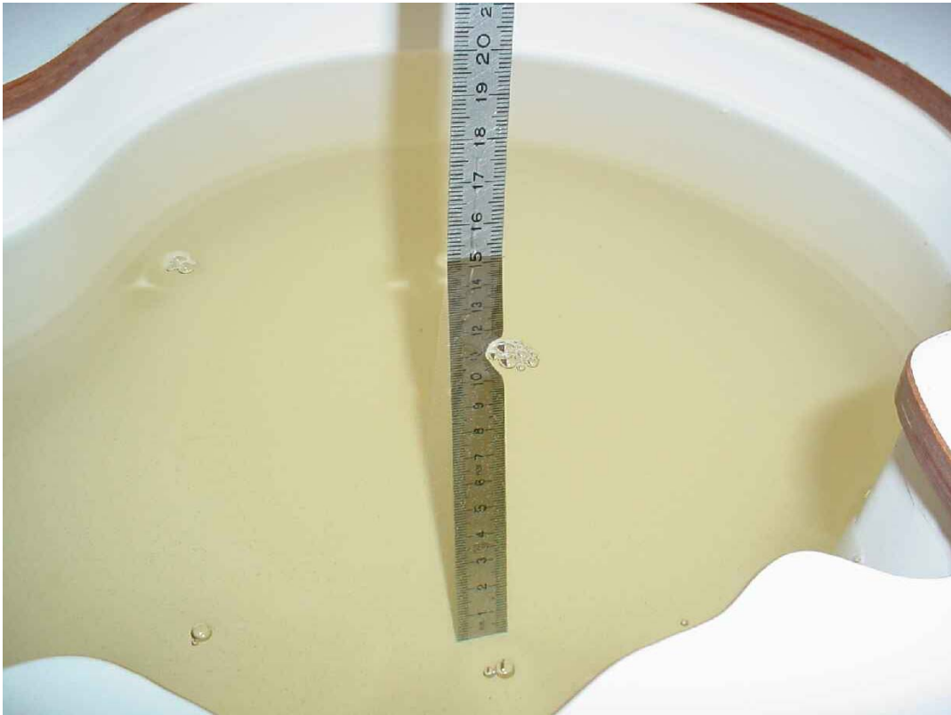
Photo 22: Liquid depth 850 MHz body simulating liquid
